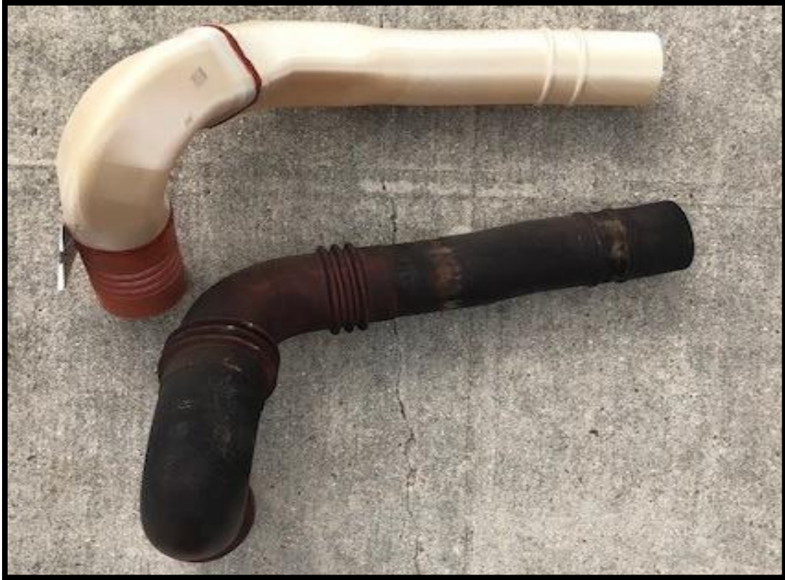
Figure 15: Top, 3D Printed Duct; Bottom, Original Duct with Rubber Boot
