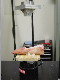
Figure 4: Mounted hind limb on dynamic loading force cell.
