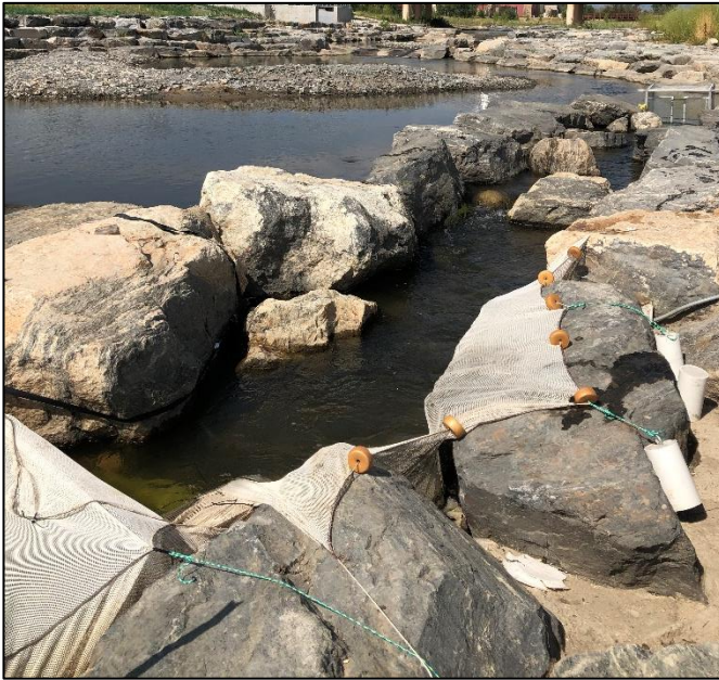
Figure 2.6- The top photo (A) shows the wingwall bypass fishway design at the Dickens Farms Natural area site. Bottom left (B) photo shows the placement of both enclosures looking in the upstream direction and bottom right (C) shows specifically the lower enclosure placement.
