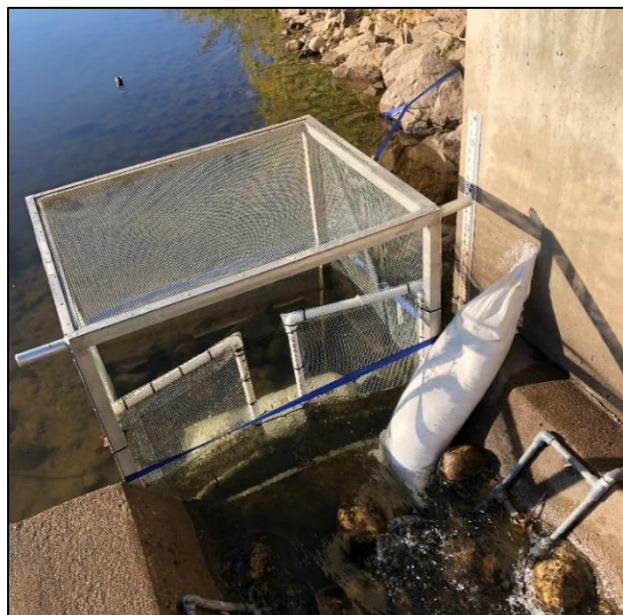
Figure 2.4- Images showing the installation of the top (at left) and bottom (at right) enclosure boxes for the trial at the FCRID site.
