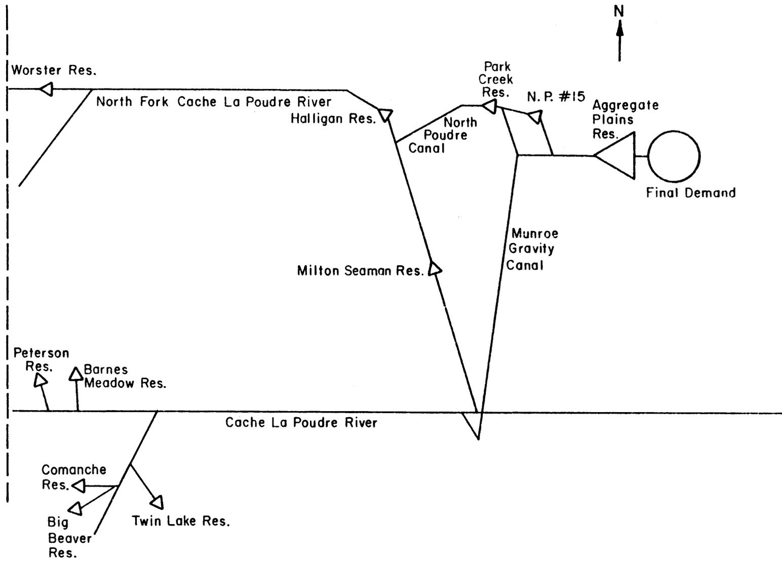
Figure S-1. Schematic of the Upper Poudre River System
