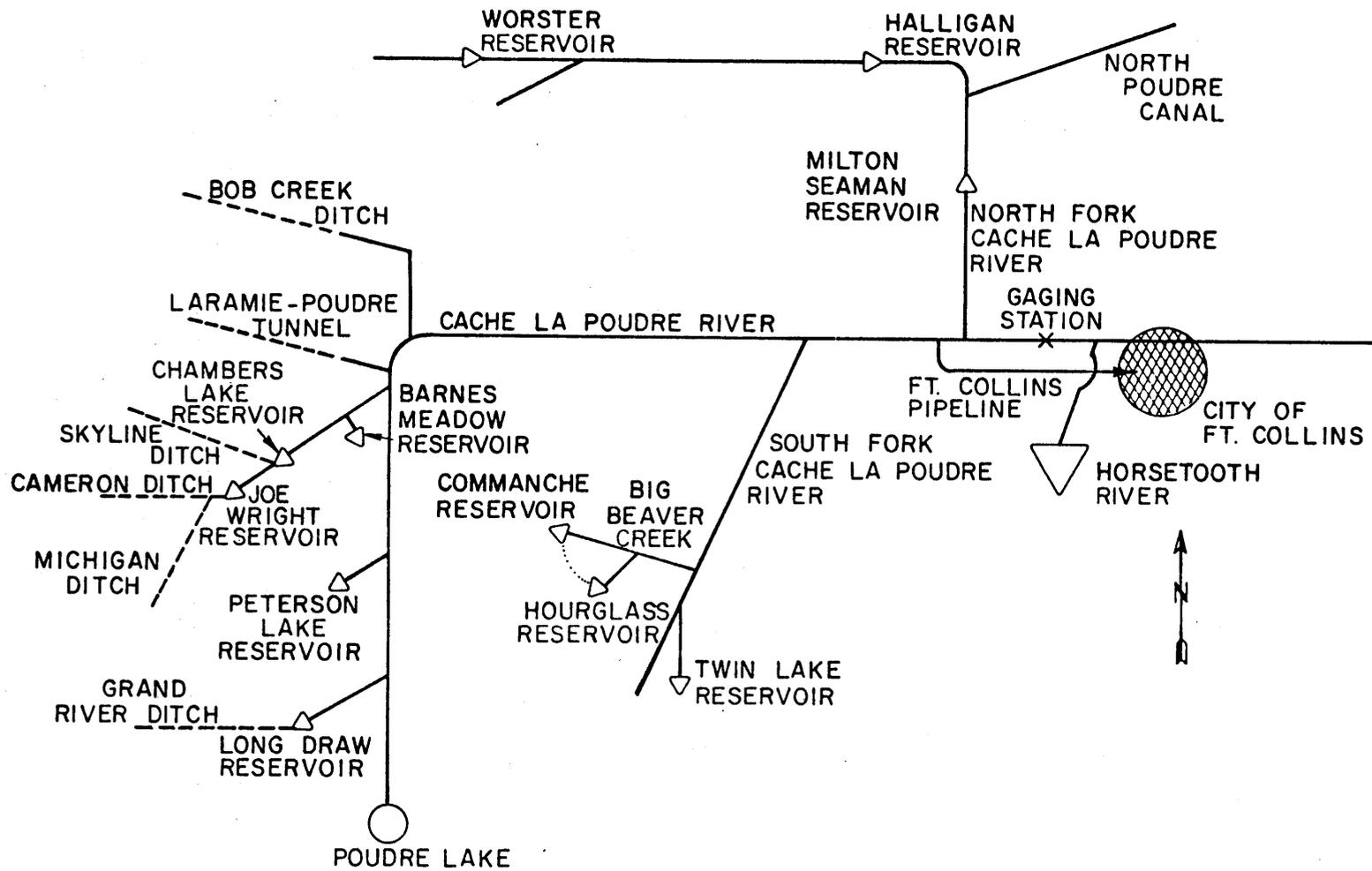
Figure 5. Schematic of the Poudre River Basin System
