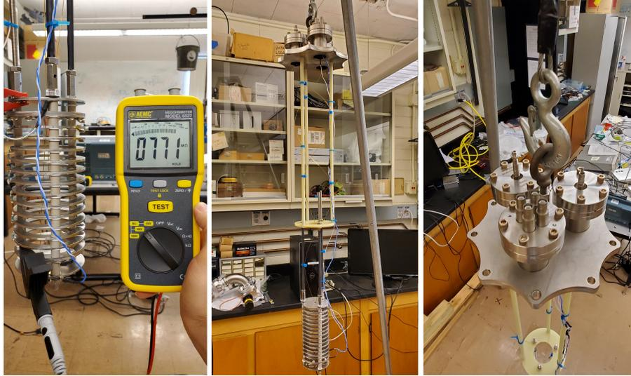
**Figure 4.5:** Purity monitor resistance test before cryostat insertion (left), full purity monitor apparatus and hanger (center), and top of purity monitor flange (right).
