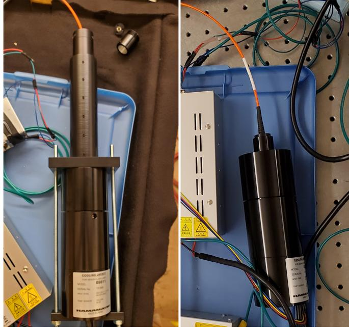
**Figure 3.4:** The two mounts for the xenon flash lamp and optical fiber. The lens tube holder (left) allows the positioning of the lenses and optical fiber relative to the flash lamp. On the right is the setup that holds the end of the optical fiber close to the glass surface of the bulb.
