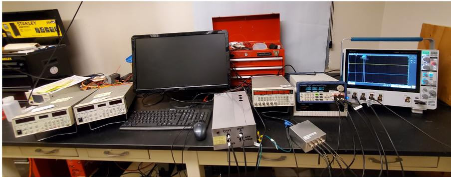
**Figure 2.7:** Purity monitor control and data acquisition station for testing the purity monitors in vacuum, gaseous argon, and LAr.
