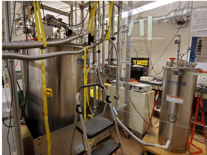
**Figure 5.5:** Experimental setup for purity monitor LAr tests.
