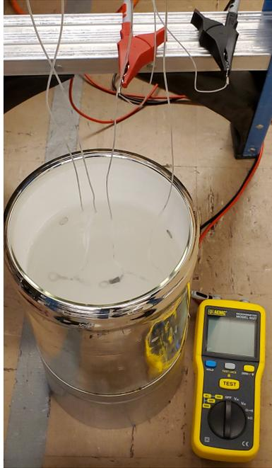
**Figure 4.7:** Resistance and robustness test of the purity monitor resistors.
