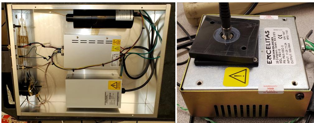
**Figure 3.2:** The Hamamatsu L7685 xenon flash lamp (left) and the Excelitas PAX-1002-3 xenon flash lamp (right).
