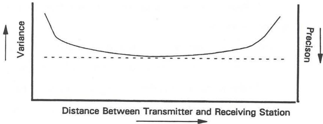
**Fig. 1.2.** Theoretical behavior of variance and precision as related to the distance between transmitter and receiving station. Solid line illustrates Pace's theory where precision increases at close and far distances. Dashed line illustrates the theory of constant precision.
