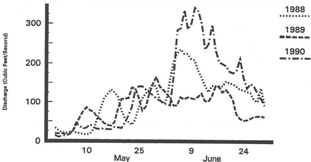
**Fig. 2.13.** Daily stream flow for Gore Creek-Minturn monitoring station for May 1 - June 30, 1988-1990. Peak flows index snow melt. Gore Creek is on the northern edge of the study site. No water diversion exists above gauging station.
