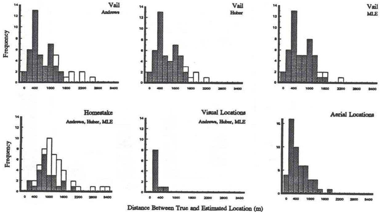
**Fig. 1.6.** Histograms of distance between true and estimated locations for ground, visual and aerial locations. Ground and visual location histograms show the performance of the Andrews Estimator, Huber Estimator and MLE. Unshaded bars are locations deleted and shaded bars are locations remaining after censoring. All 3 estimators produced the same histograms for Homestake and the visual locations. Unshaded bars are locations deleted after censoring.
