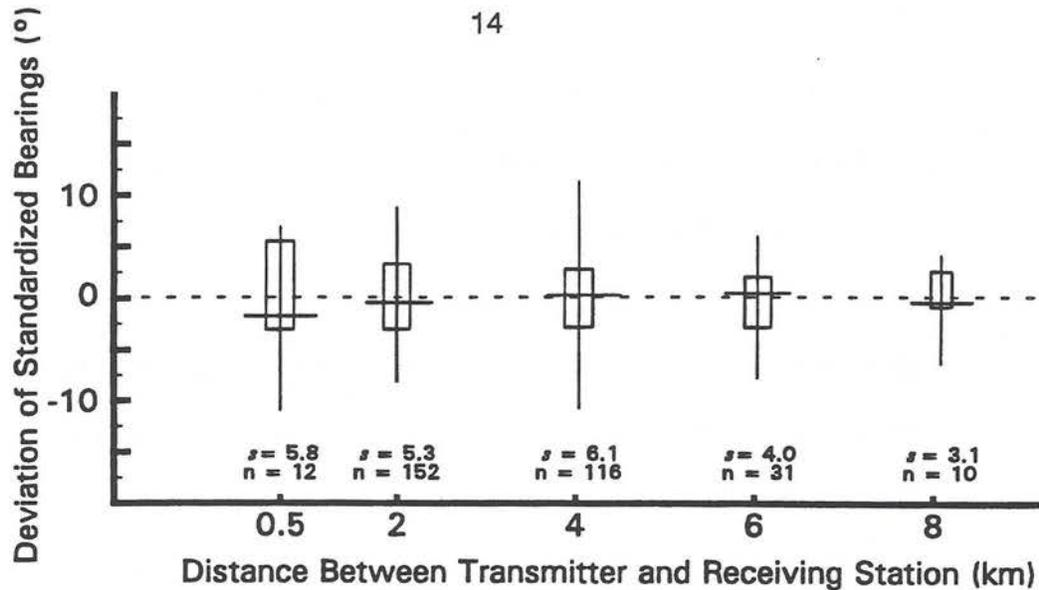
**Fig. 1.4.** Precision of standardized telemetry bearings as related to distance between transmitter and receiving station. Horizontal line marks median, upper and lower box lines mark 75% and 25% quantile, respectively, and upper and lower points of each vertical line mark 95% and 5% quantile, respectively. I detected no difference overall ( $P = 0.13$ ), but a difference was detected when bearings were pooled for the first 3 groups and compared to the later 2 groups ( $P = 0.02$ ).
