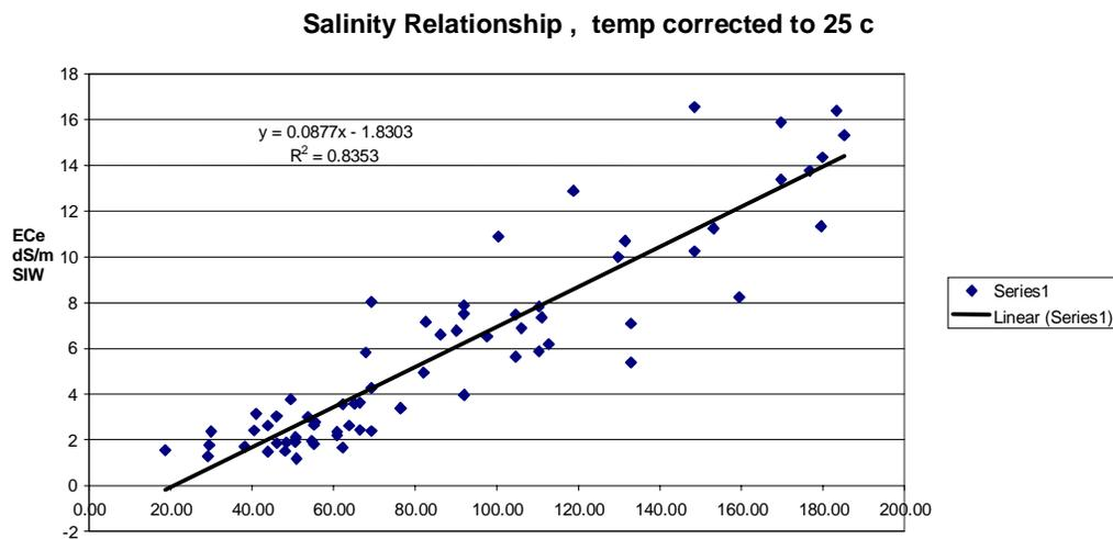
Figure 1. Regression equation relating EM<sub>v</sub> and EC<sub>e</sub>.
