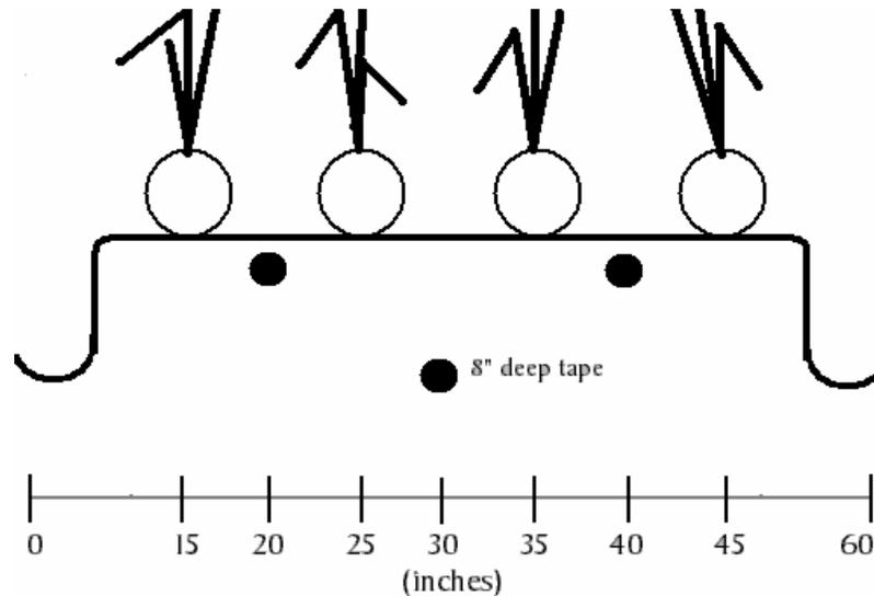
**Figure 1:** Comparison of drip line placement for onion production; the standard single line placed 8 inches deep in the center of the bed and the more efficient configuration of two lines placed at a shallower depth.
