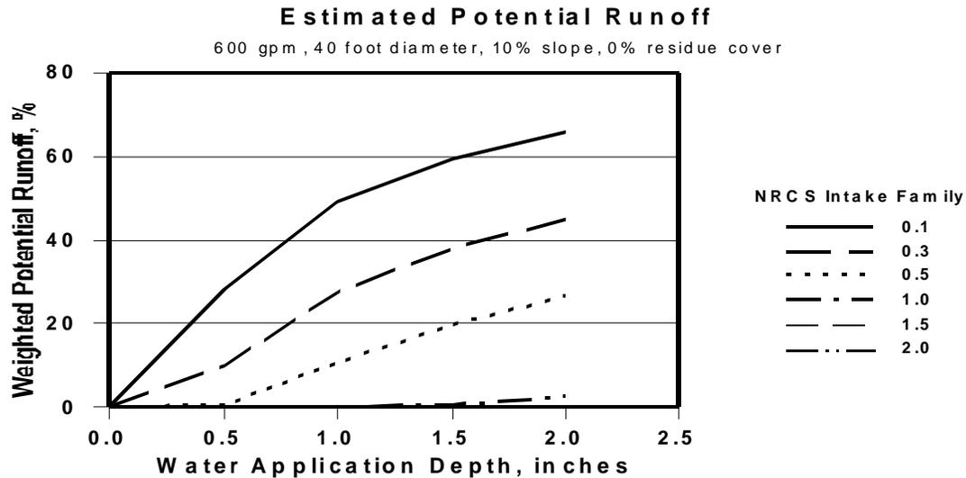
**Figure 4.** Effect of soil intake family and water application depth on weighted potential runoff for a 1320 foot center pivot with a sprinkler package wetted diameter of 40 feet and a flow rate of 600 gpm.
