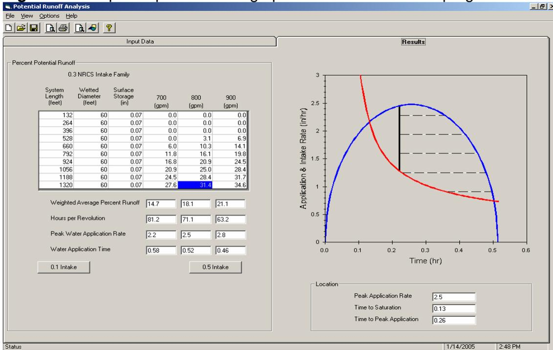
Program output includes a table presenting potential runoff for 10 positions along the system and the weighted potential runoff for the entire field. Output generated for a system with inputs of 1320 foot system, 800 gpm, 1.0 inch
