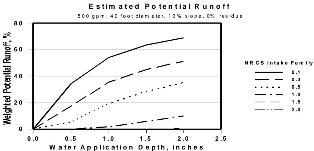
**Figure 3.** Effect of soil intake family and water application depth on weighted potential runoff for a 1320 foot center pivot with a sprinkler package wetted diameter of 40 feet and a flow rate of 800 gpm.
