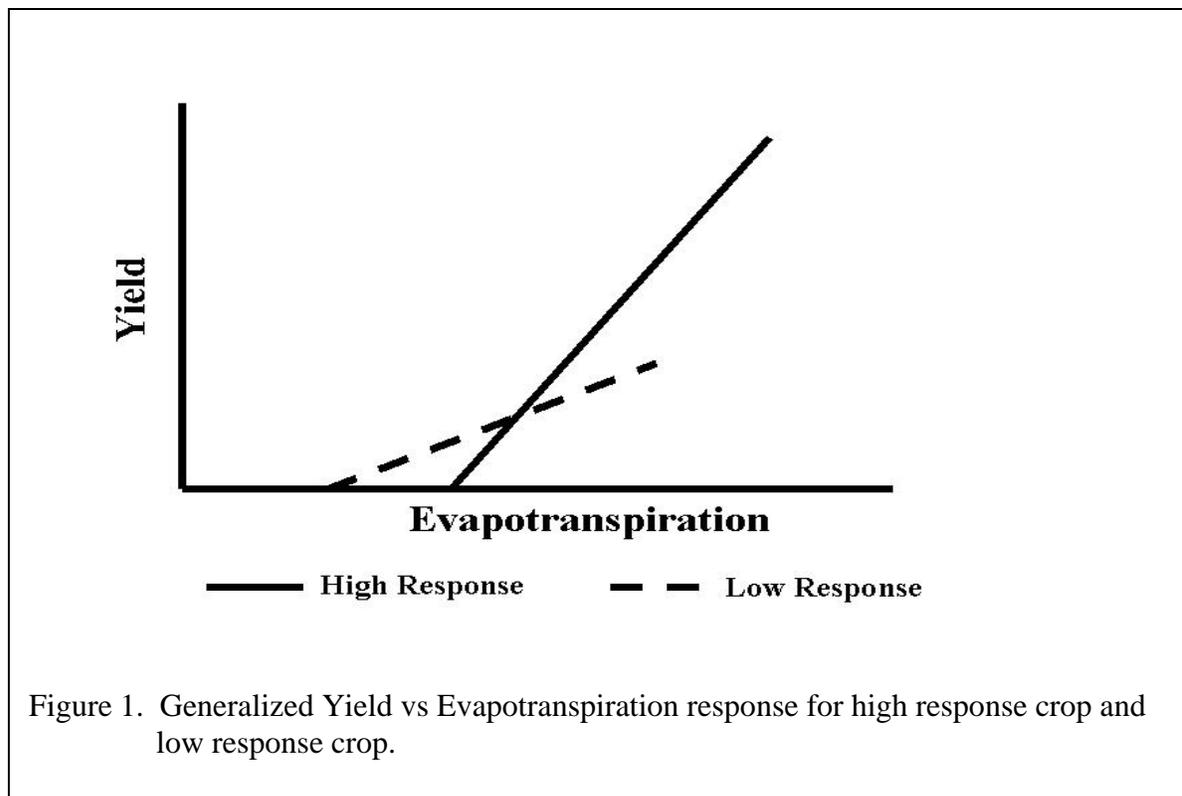
Figure 1. Generalized Yield vs Evapotranspiration response for high response crop and low response crop.
