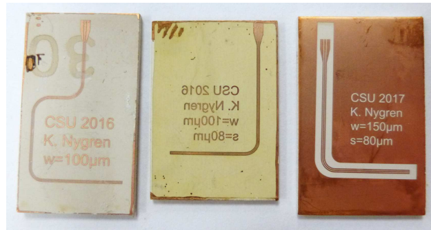
Figure 7.3: Antennas made for \text{VO}_2 sample excitation. Iterations 1, 2, and 3 (left to right).
