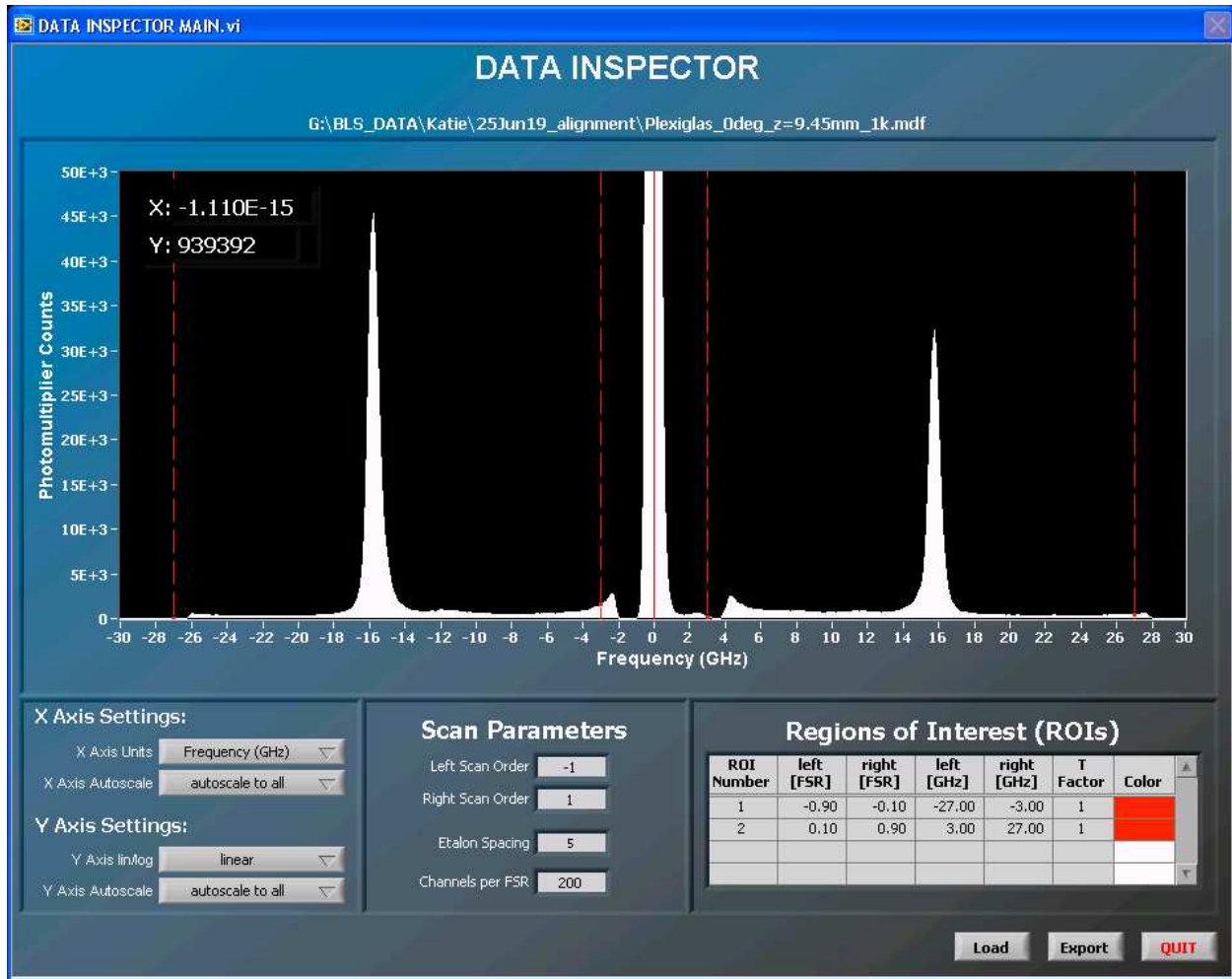
Figure 3.6: TFPDAS4 software window showing a data set from a transparent acrylic plastic like Plexiglas after \sim 6 minutes of data collection time. The central white peak (at 0 GHz) is the signal from the reference beam, whereas the white peaks at \pm 15.7 GHz are the signal from the acrylic sample. The red dashed lines form the outside edges of two regions of interest (ROI) where the sample data is collected. These red lines denote where the double should switch between the sample beam and the reference beam or vice versa. The small peaks around -2.5 GHz and +4.5 GHz are bleed-over signal from the elastically scattered light that was not completely blocked by the double shutter. The intensity of the acrylic data peaks can be used to determine quality of interferometer alignment.
