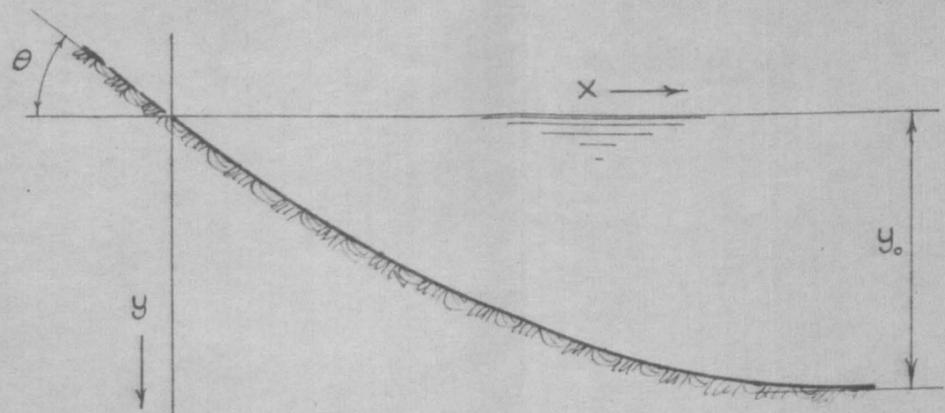
$\theta$  = Angle of repose of saturated bed material
