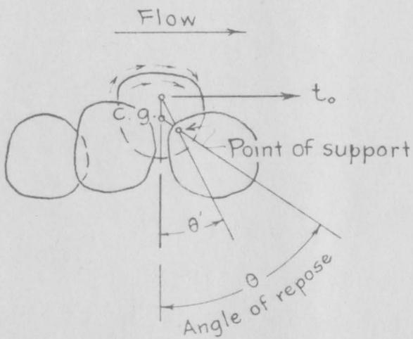
Fig. 2.—Equilibrium of an individual particle on a horizontal plane when the surface drag is of major importance.
