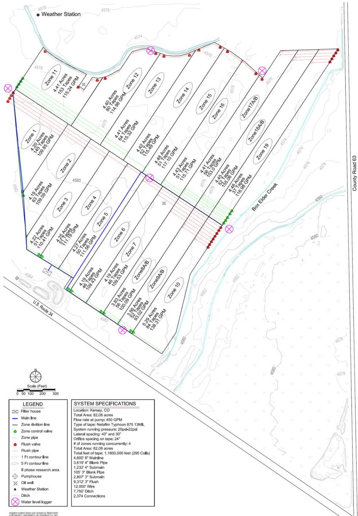
Figure 2.1. SIEP site map of the experimental field zones and irrigation system specifications.
