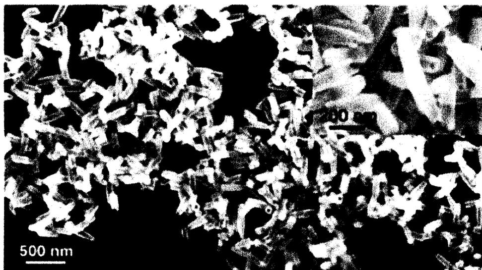
**Figure 1.6.** SEM images of the single crystalline Fe<sub>2</sub>O<sub>3</sub> nanotubes formed by hydrothermal synthesis.<sup>35</sup>
