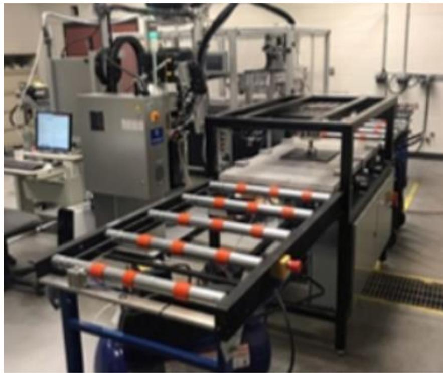
Figure 13: Image of pneumatic press utilized at MEL.
