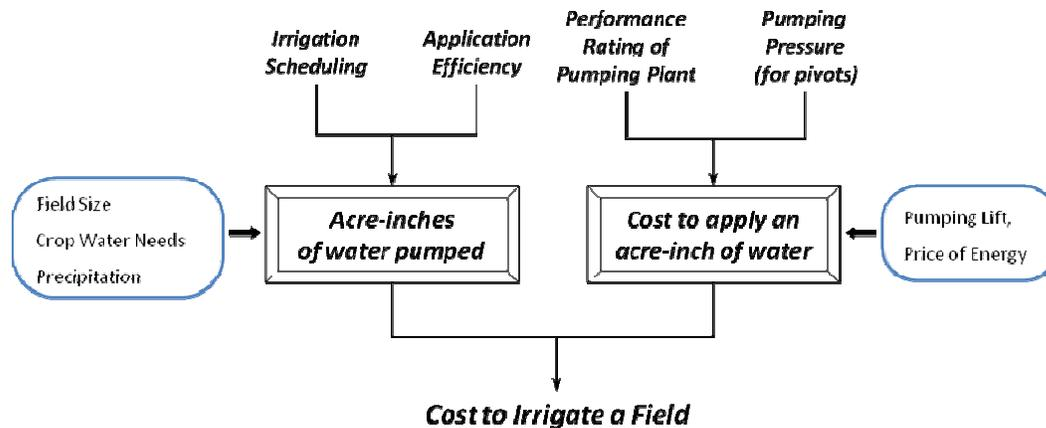
Figure 1. Diagram of factors affecting irrigation pumping costs
