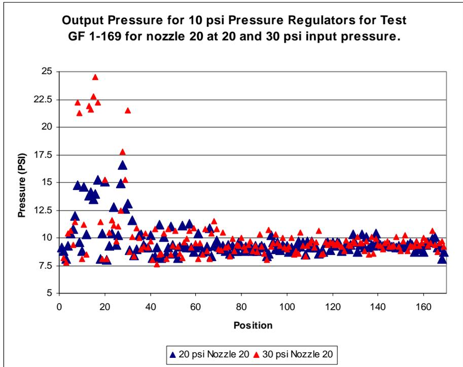
Figure 8. Output pressure of 169 pressure regulators tested at 20 and 30 psi input pressure. Tests GF 1-169.
