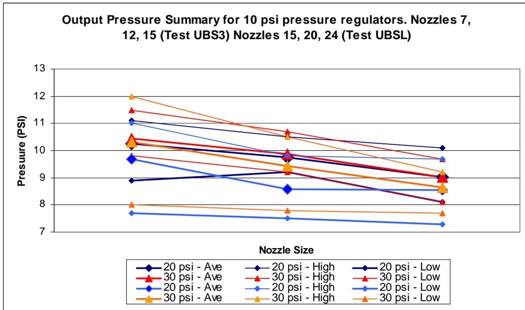
Figure 6. Average, high and low output pressures for 10 psi pressure regulators for Tests UB S3 and LS.
