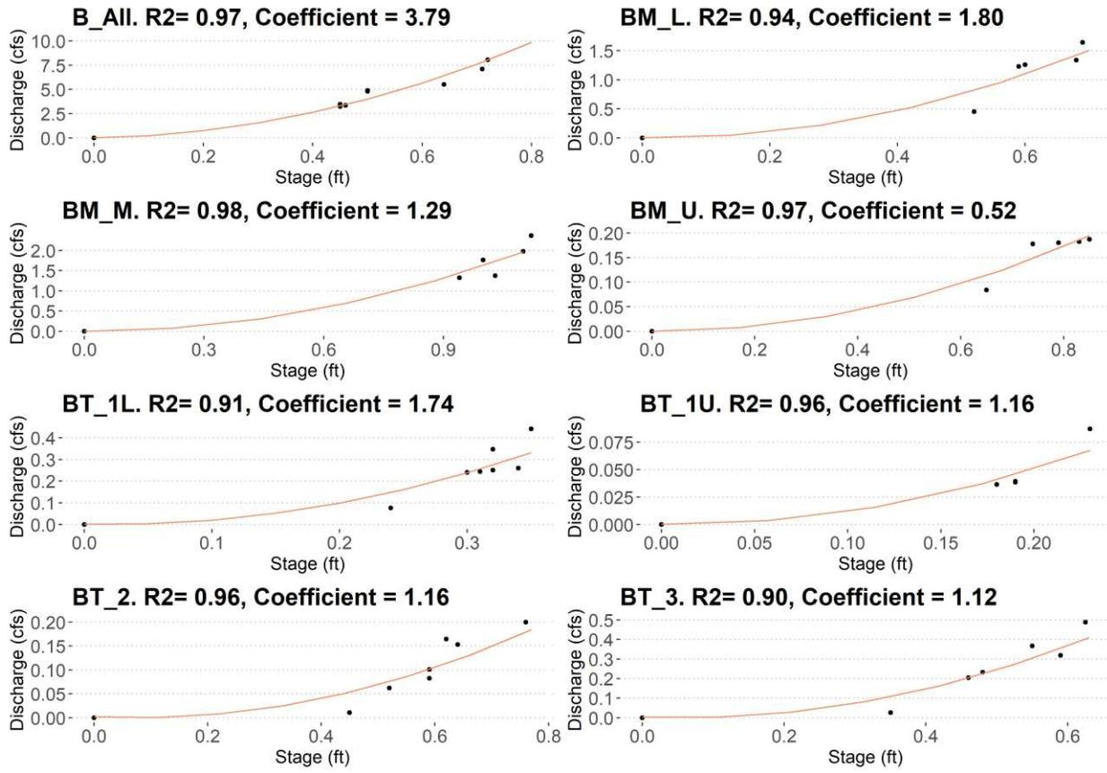
Figure A2a. Relationship between manual discharge measurements and stream stage readings. Coefficient of determination value and  $\beta$  values is also included.
