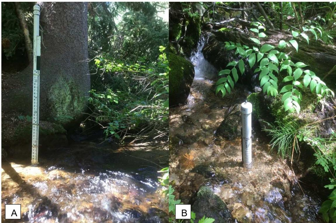
*Figure 9. Stream stage installation types, a) stilling well with stage plate and b) modified mini stilling well.*
