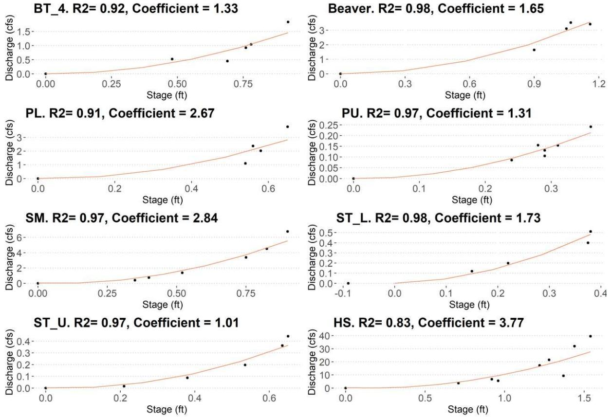
Figure A2b. Relationship between manual discharge measurements and stream stage readings. Coefficient of determination value and  $\beta$  values is also included.
