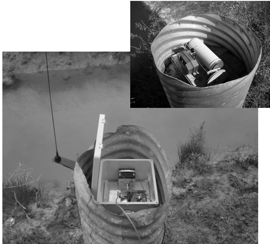
Figure 3. In several cases, the existing Stevens recorder was replaced with a SCADA RTU with the replacement electronics costing less, by comparison, than a new replacement Stevens recorder.
