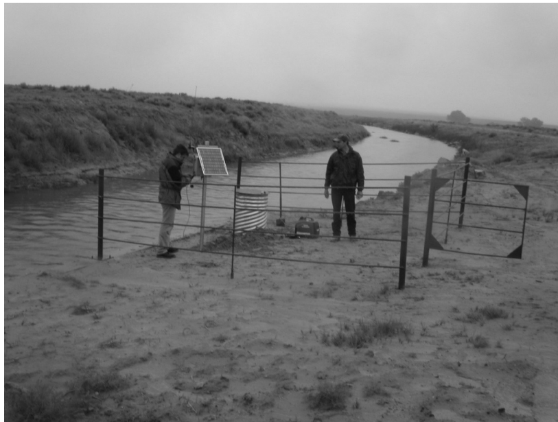
Figure 1. This installation of an RTU is on a rated section of the main canal. A small generator was used for incidental power needs during installation. A fence protects the equipment from grazing cattle.
