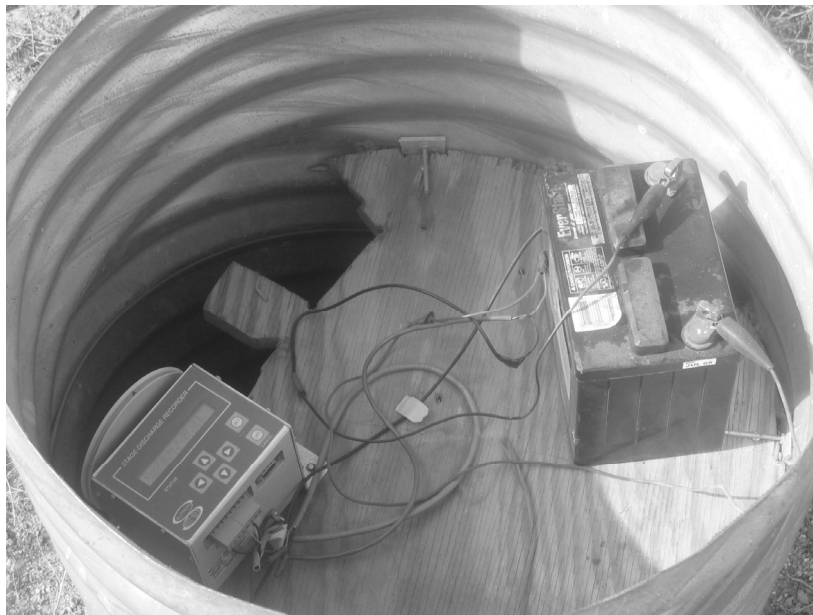
Figure 4. Several WSL sensors were tried before focusing on a float and wheel arrangement that has proved to meet expectations for accuracy.
