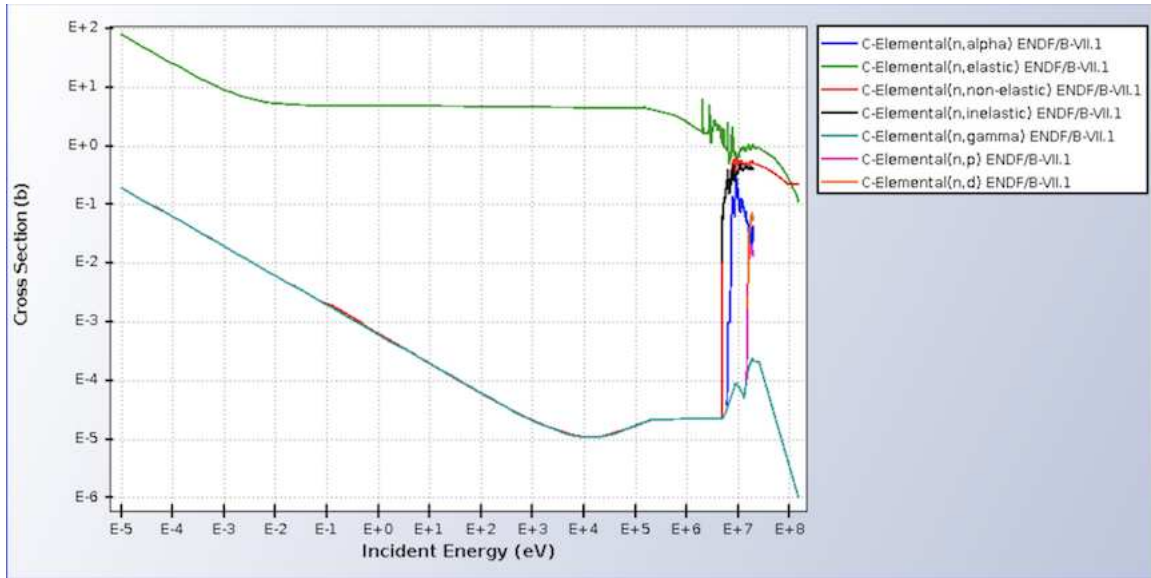
Figure 2.5: Cross section measurements for a neutron with carbon target as a function of incident neutron energy. For lower energies, elastic is the most dominant mechanism. For neutron energies greater than 1 MeV, other processes begin to turn on. Plot from ENDF [4].
