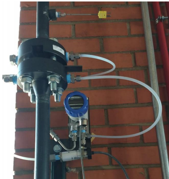
Figure Appendix - 6. Orifice plate flow measurement system. Natural gas mass flow measurement. Identical set up used on EGR cart, and Air flow measurement.
