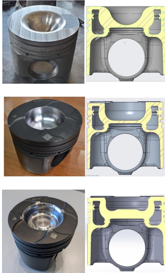
Figure 30. Top: Prototype A piston. CR 16; Middle: Prototype B piston. CR 13.3:1; Bottom: Prototype C piston. CR 15:1.
