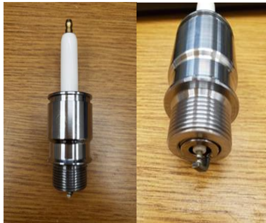
Figure Appendix - 4 Bosch MR3DII360 spark plug and spark plug insert as used during the baseline testing.
