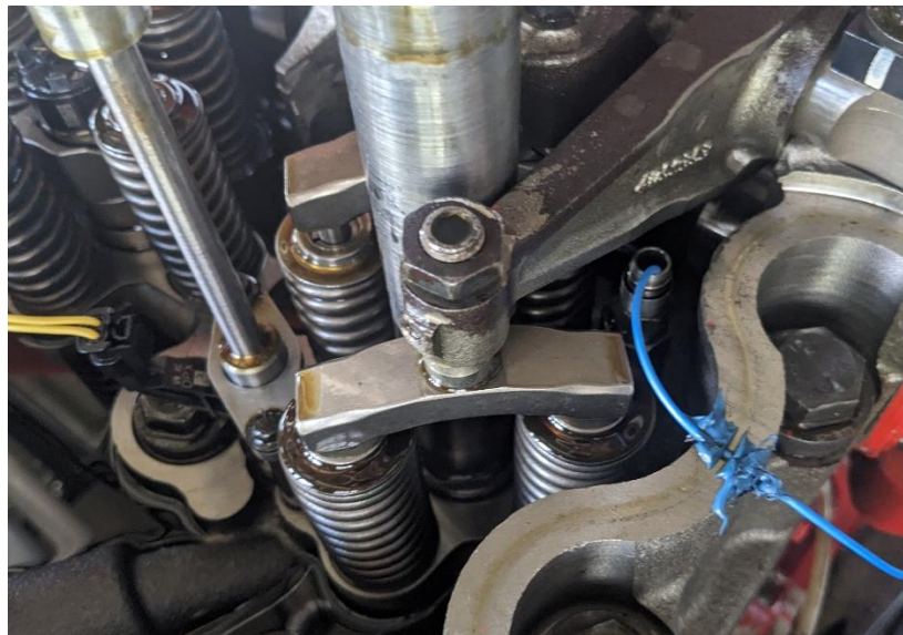
Figure 72. X15 SCE head. AVL and direct injector location.
