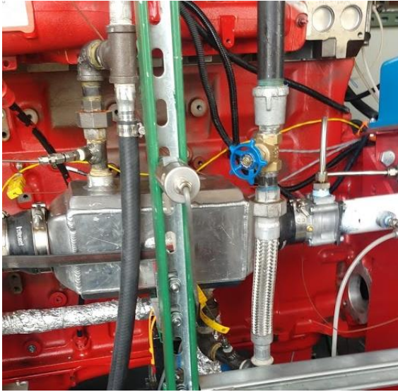
Figure Appendix - 3. Intake heat exchanger and schematic for Intake temperature control.
