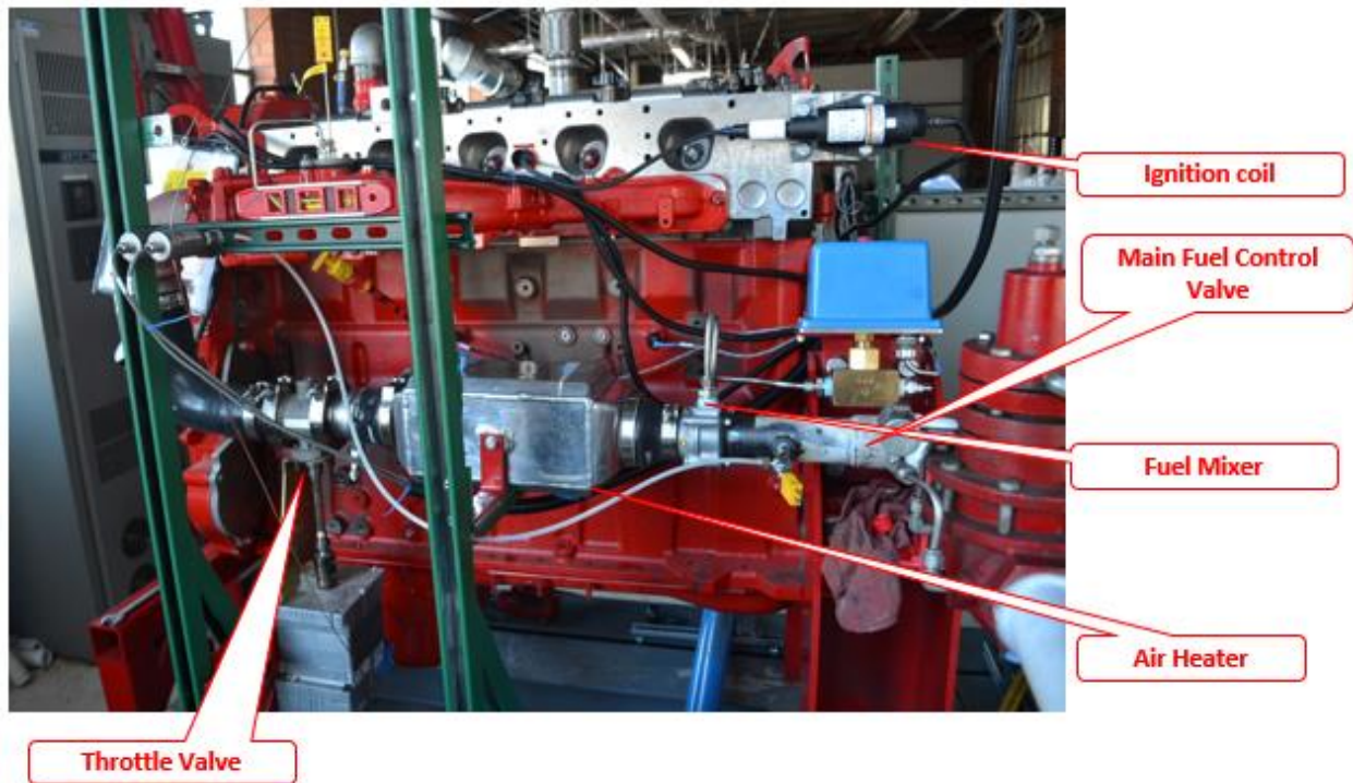
Figure Appendix - 1 Cummins X15 SCE intake system.
