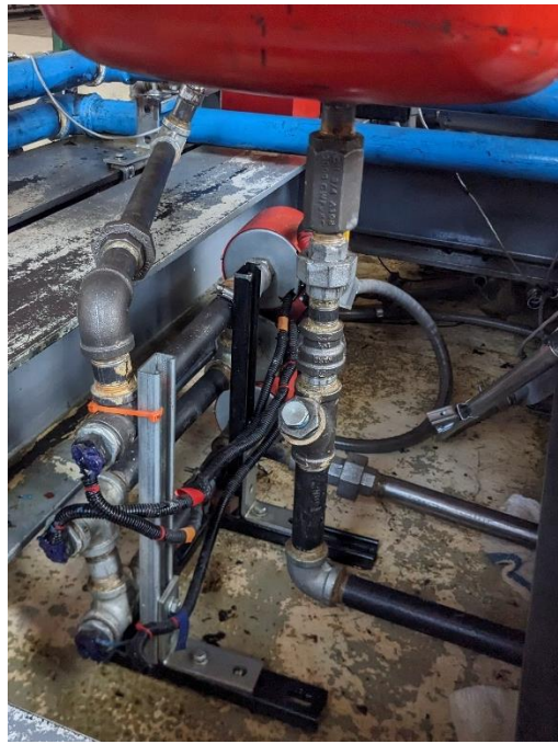
Figure 12. Oil heater system installed on the SEC X15 engine.
