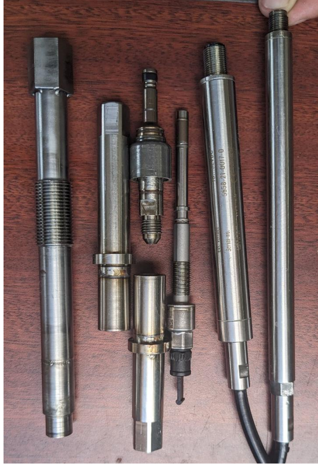
Figure 70. Sensors tested and adapters. From left to right: adapter for IMES sensor in original in-cylinder pressure location, adapter IMES sensor in DI location, Adapter CAT sensor on DI location, CAT sensor, IMES sensor amplifier, and sensor body.
