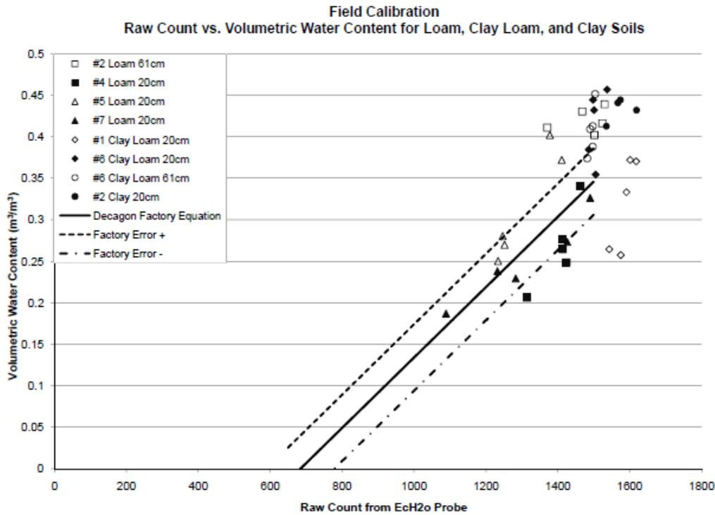
Figure 5. Field Calibration Compared to Factory Calibration Curve for Loam, Clay Loam, and Clay Soils
