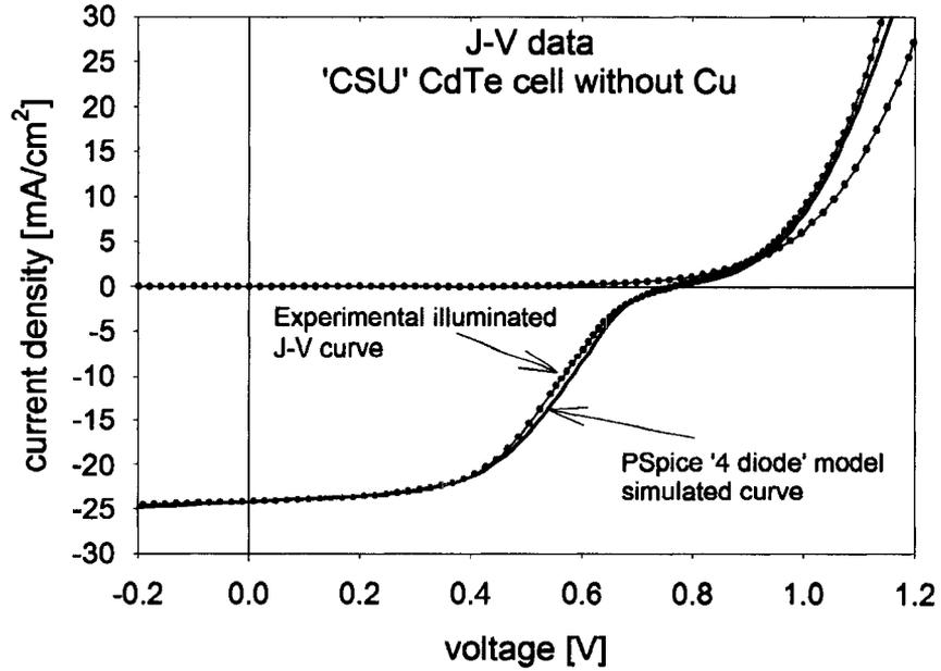
Figure 3.14: Nonstandard J-V behavior which is not explained by the two-diode model of back-barrier induced rollover, can be closely fit (green curve) by assuming non-uniformity of the device performance and modeling with parallel circuit branches representing well-behaved, and rollover-type areas coexistent on the same device.
