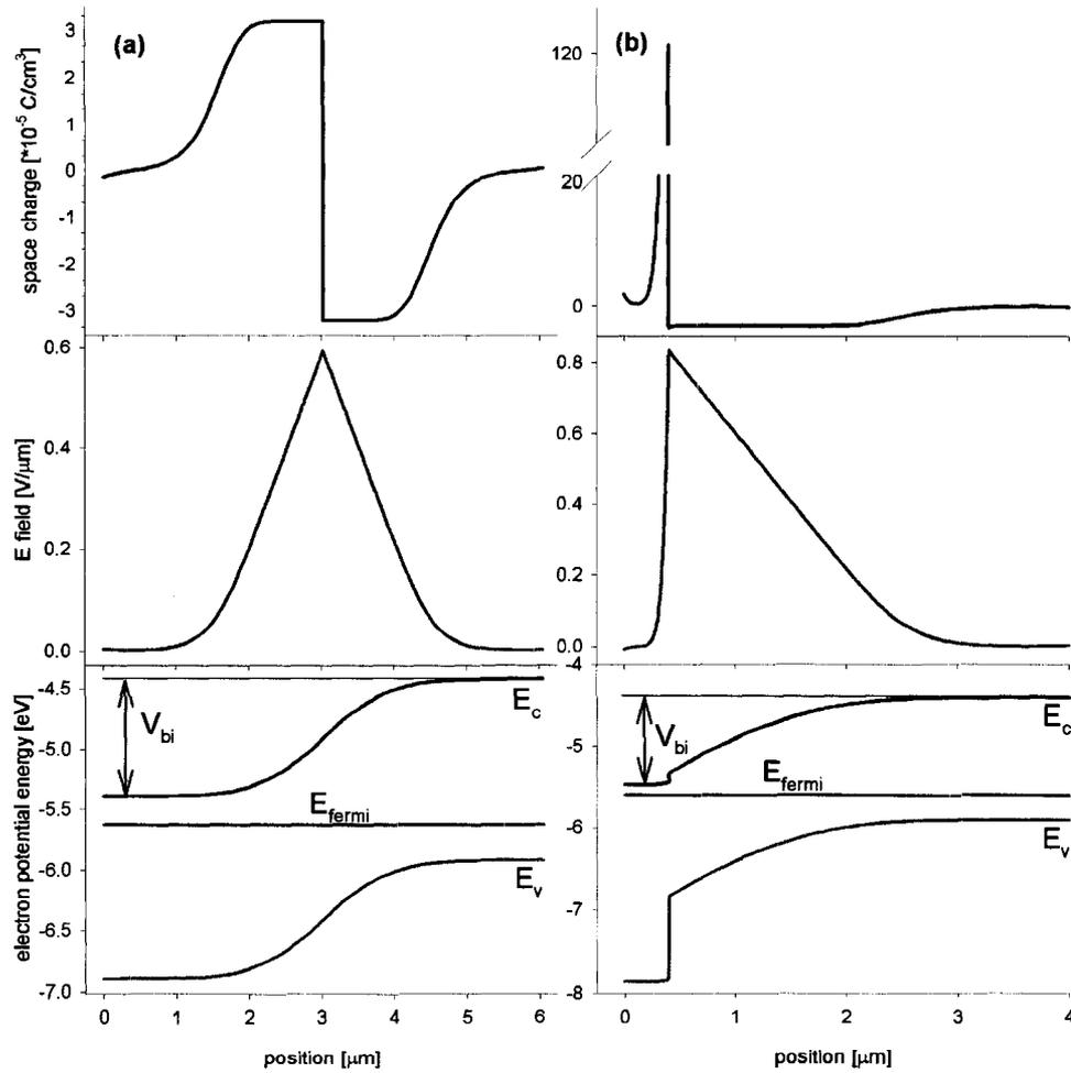
Figure 2.3: Charge, electric field, and energy bands of a (a) generic homojunction with equal n- and p-type doping and (b) a heterojunction with typical parameters for CdS (n-type, left side) and CdTe (p-type, right side)
