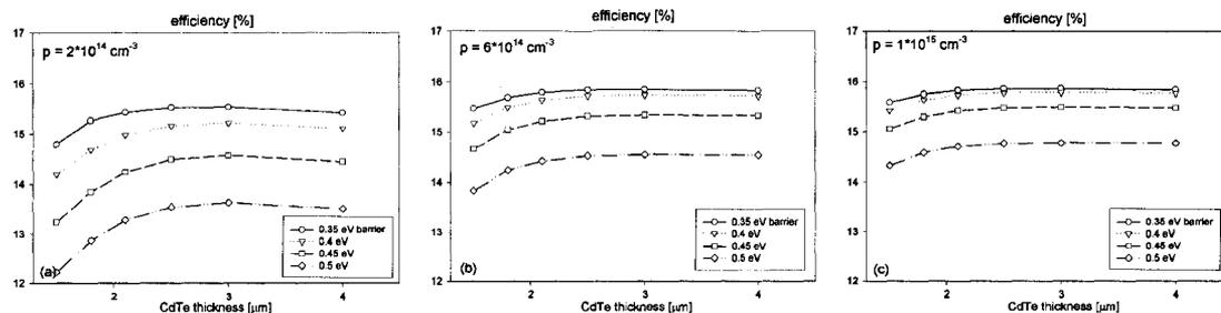
Figure 4.2: The efficiency as a function of absorber thickness for three carrier densities and multiple values of the back-contact barrier height. Efficiency is highest when the absorber is thick enough to separate the front and back depletion regions, but can be reduced if the CdTe is thick enough that collection suffers.
