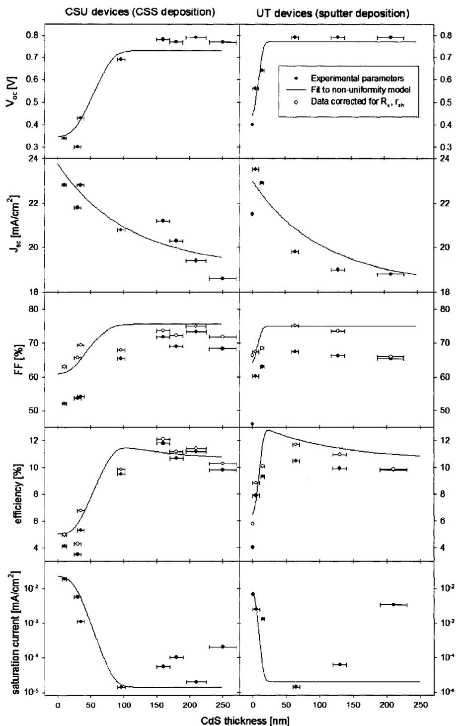
Figure 5.9: First and second level parameters from J-V measurement plotted for CdS thickness inferred from QE. Since the non-uniformity model applied does not include the effects of series and shunt resistances, the FF and efficiency data are plotted without (filled points) and with (open points) series and shunt resistance correction.
