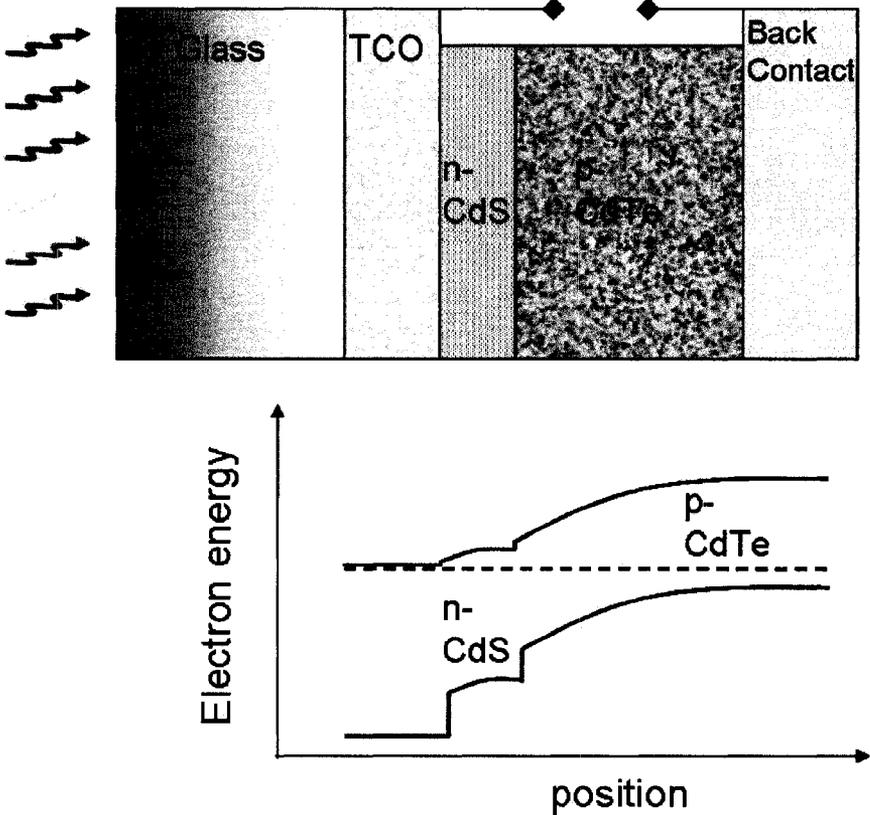
Figure 1.4: Ideally, the deposited layers of the solar cell form a large-area photosensitive diode. In practice, many non-idealities exist, including parasitic resistances and non-uniform physical and electrical properties. (layer thicknesses exaggerated)
