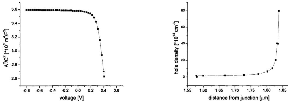
Figure 2.11: A thin absorber might be fully depleted, so that the depletion width cannot respond to voltage bias. Apparent carrier densities are often skewed in this situation.
