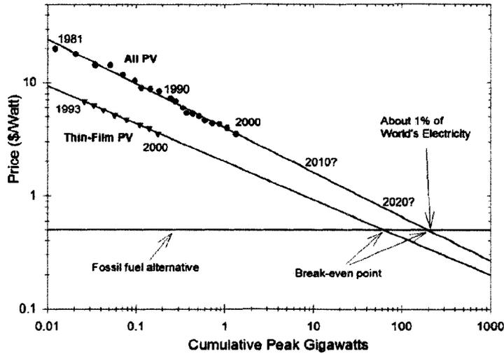
Figure 1.3: Price comparison for thin-film and Si photovoltaics. For equal production volume, thin-film PV delivers significant cost advantages. Figure reproduced from [5].
