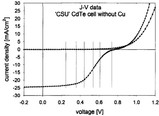
Figure 3.11: Experimental J-V curves for a ‘CSU’ device without Cu in the back contact. Voltage bias levels for LBIC measurements are also indicated.
