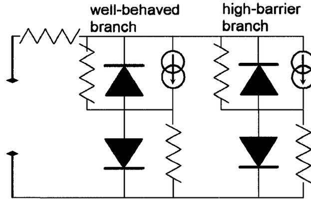
Figure 3.8: In the generalized equivalent circuit for a device with non-uniformities, the contributions from non-ideal components (back-contact barriers and main-junction variations) are averaged into a single set of parameters for the ‘weak branch’. The strong branch behaves much like the circuit from 3.2 with a very low barrier.
