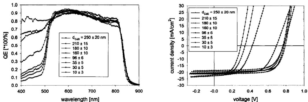
Figure 5.4: CdS layer thickness is inferred from QE data in the  $400 < \lambda < 500$  nm range. When the CdS layer is thinner, photocurrent increases slightly. However, below about 100-nm layer thickness,  $V_{oc}$  and FF suffer more dramatically, reducing overall device performance. The likely culprit of reduced performance is transition to performance dominated by the weaker  $\text{SnO}_2/\text{CdTe}$  junction.
