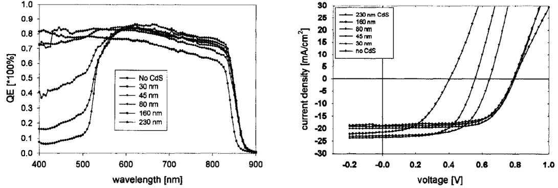
Figure 5.6:  $V_{oc}$  is virtually constant for the sputtered devices for CdS thicknesses down to 80 nm (as deposited). All devices with high CdS-region QE have reduced  $V_{oc}$  and FF.
