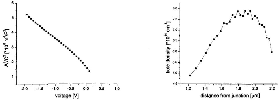
Figure 2.10:  $A^2/C^2$  for a well-behaved device decreases with increasing voltage because the depletion width reduces with bias. The carrier density is obtained from the slope of the  $A^2/C^2$  graph.
