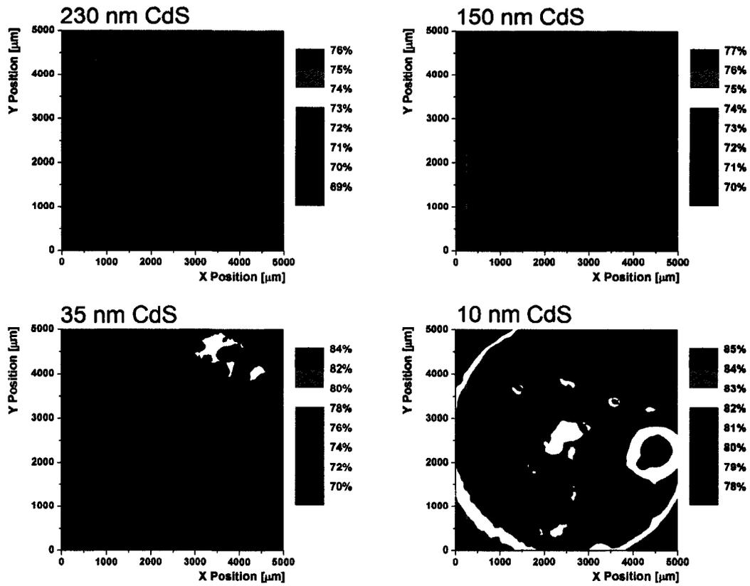
Figure 5.5: Low-resolution LBIC data for representative thick (top) and thin (bottom)-CdS layer devices. The variations obvious in thin-CdS devices may be indicative of  $\text{SnO}_2/\text{CdTe}$  junction regions in parallel with CdS/CdTe.
