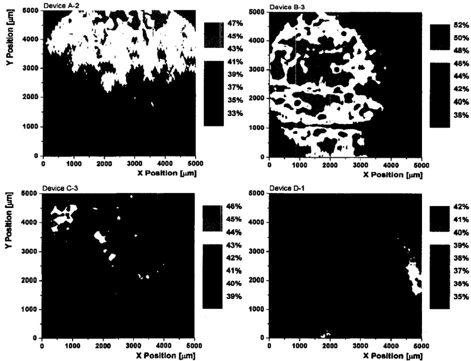
Figure 3.6: The development of non-uniform photocurrent collection with increasing voltage shows that much greater spatial variations exist in the collection of cells without Cu-containing contacts, than in those with Cu. Variable back-contact barrier influence is the most logical culprit, given the expected influence of the Cu. Bias levels were chosen so that  $QE_{bias} \sim QE_{sc}/2$
