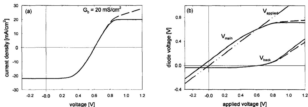
Figure 3.3: Simulated current-voltage curves (a) and voltage distribution (b) for the equivalent circuit of figure 3.2 with back-contact leakage conductance of 0 (solid lines) and 20 (dashed lines)  $\text{mS/cm}^2$ . The back diode has a saturation current of  $20 \text{ mA/cm}^2$ , corresponding to a barrier height of  $0.436 \text{ eV}$ .
