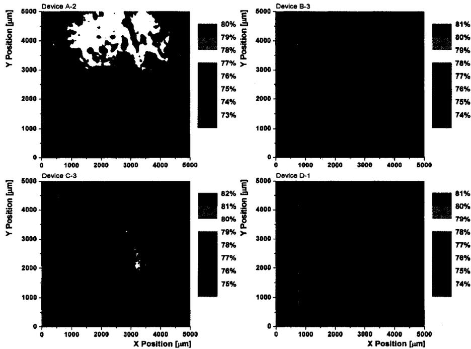
Figure 3.5: Regardless of  $\text{CdCl}_2$  treatment conditions, the addition of Cu at the back contact improves the uniformity of photocurrent collection. All scans at zero voltage bias.
