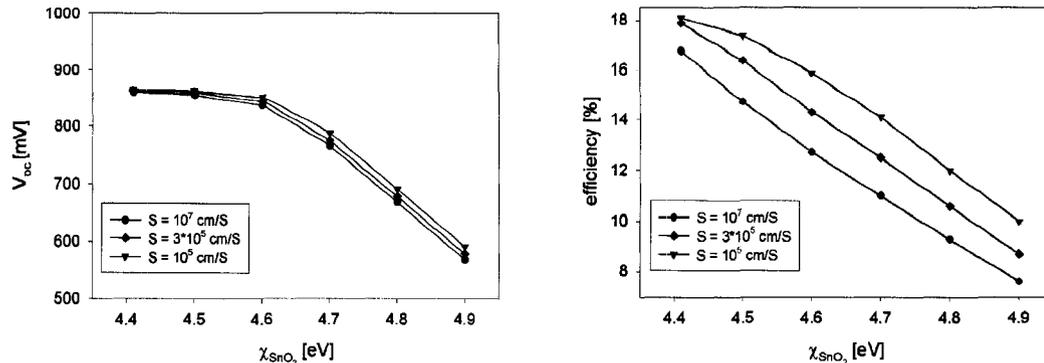
Figure 5.3: Simulation results for  $V_{oc}$  and  $\eta$  as a function of  $SnO_2$  electron affinity and various values of the interface recombination velocity.  $V_{oc}$  depends strongly on the  $SnO_2$  electron affinity for  $SnO_2/CdTe$  junctions. Efficiency benefits from improved FF and current collection due to low recombination velocity, even at small offset values.
