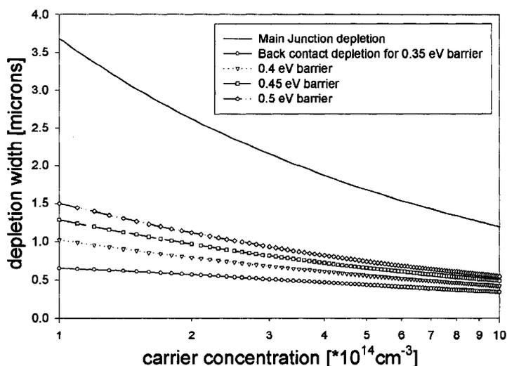
Figure 4.1: An absorber layer with thickness greater than the combined depletion widths from the front and back regions should be less susceptible to influence from non-uniformities in the back-contact
