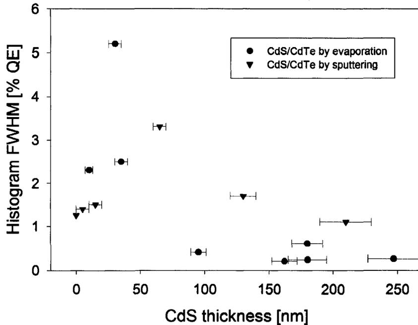
Figure 5.8: The peak in non-uniformity for devices with CdS thickness between about 30 and 60 nm coincides with the transition region from SnO<sub>2</sub>/CdTe to CdS/CdTe junction inferred from J-V data. The critical CdS thickness for evaporated devices based on SnO<sub>2</sub>-coated window glass is concluded to be in the range of 30 nm.
