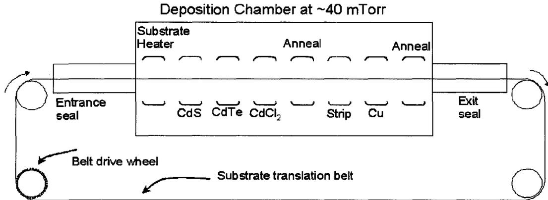
Figure 3.1: The all-in-one deposition process conceived at Colorado State enables fabrication of high-efficiency PV devices using a minimum of materials, processing complication, and space.
