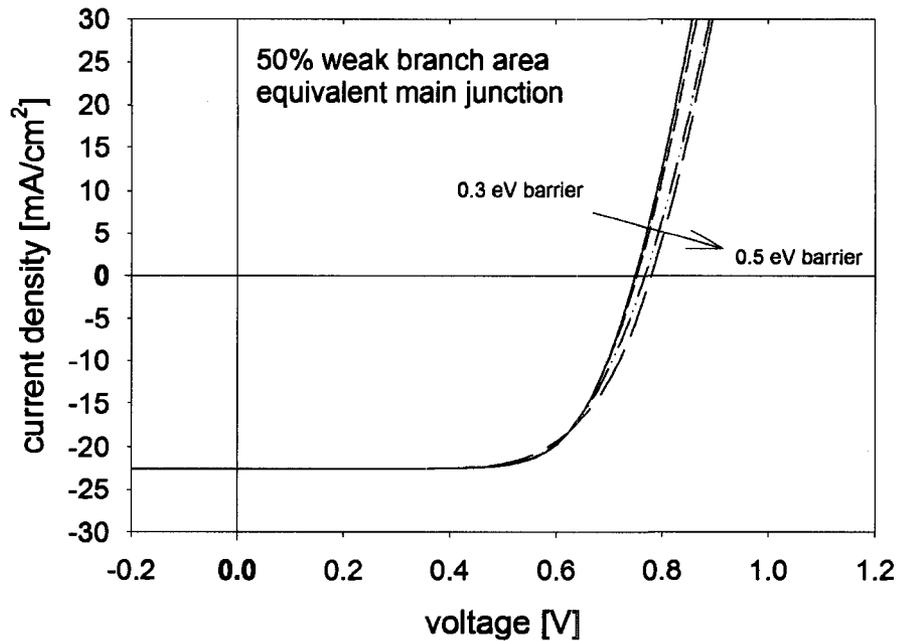
Figure 3.9: The five curves which nearly overlap are the result of the equivalent circuit of figure 3.8. The barrier heights simulated are 0.3, 0.35, 0.4, 0.45 and 0.5 eV. For the highest barriers, there are small deviations in FF and  $V_{oc}$ .
