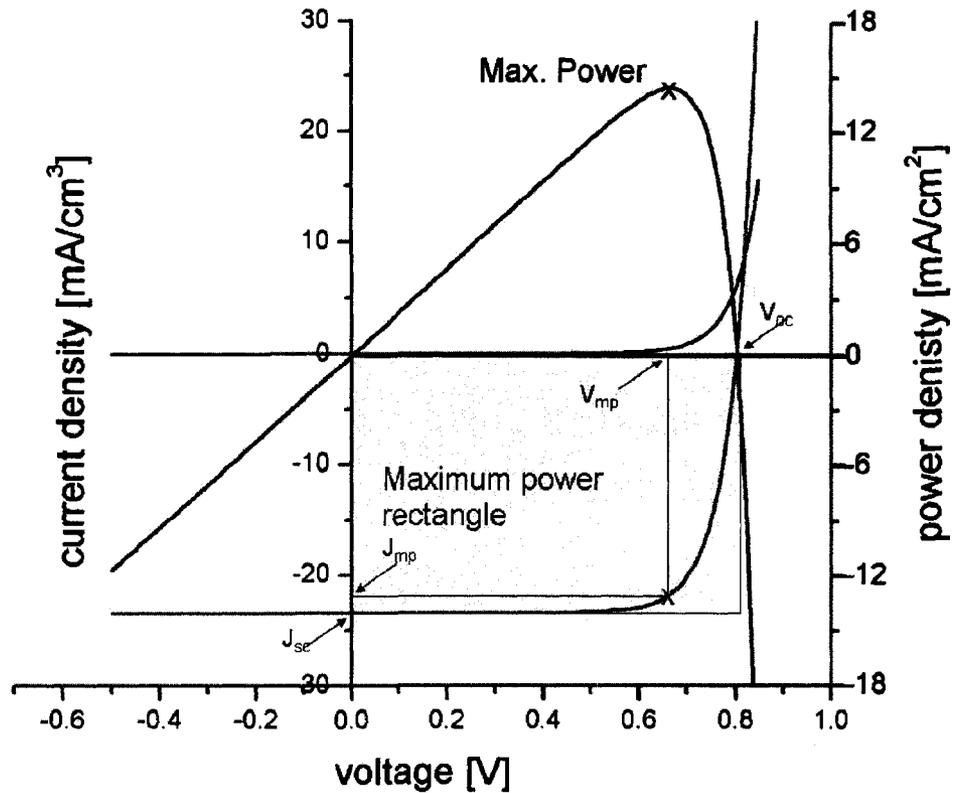
Figure 2.6: A typical J-V curve in dark (black) and light (red) for a CdTe thin-film solar cell. The power output (blue, right hand axis) is the figure of primary interest for solar cell efficiency.
