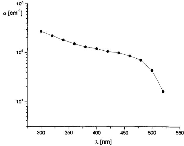
Figure 5.1: Absorption data for thin-film CdS [50]. The absorption coefficient in the range 2.4 - 3.0 eV allows a good estimate of the CdS layer thickness based on the QE data in the 400-500 nm range.
