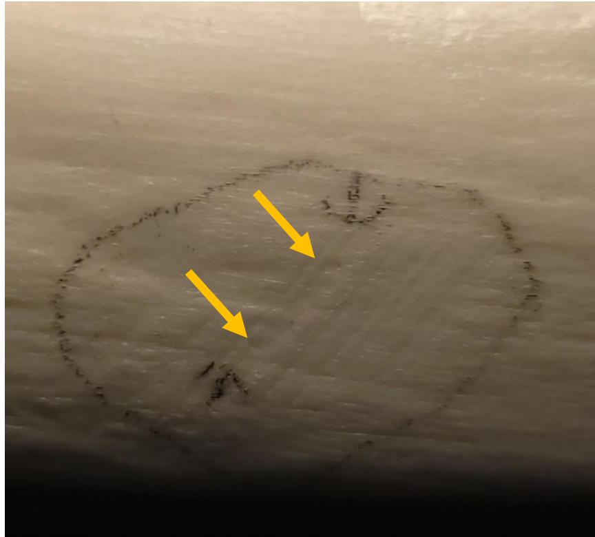
Figure 26 Impact pits indicated by the arrows
