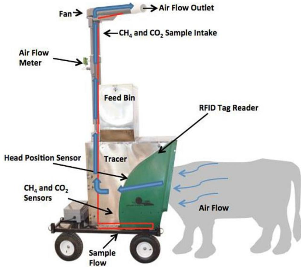
Figure 2. Components of the Automated Head-Chamber System (AHCS) used for measuring enteric emissions production (Altered from Hristov et al., 2015).
