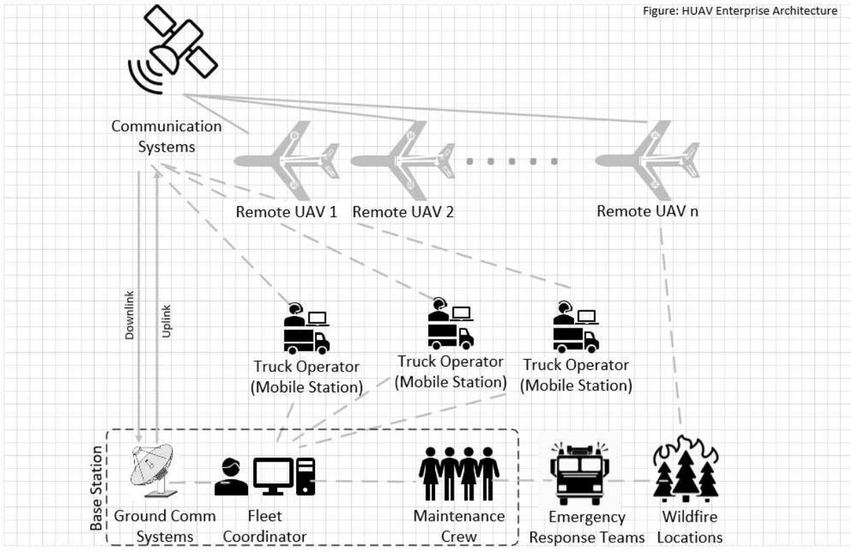
**Figure 26: H-UAV Enterprise Architecture**
