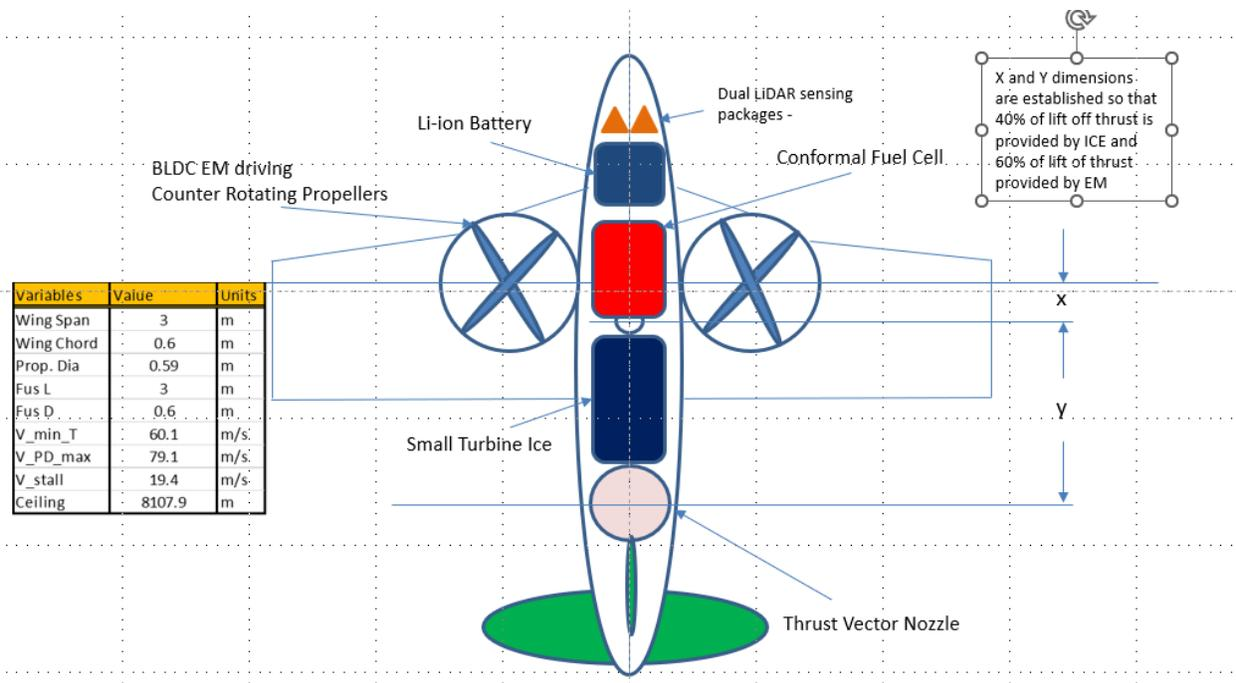
Figure 22: Initial H-UAV System Layout
