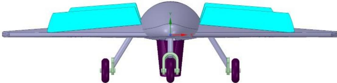
Figure 23: H-UAV Landing Configuration
