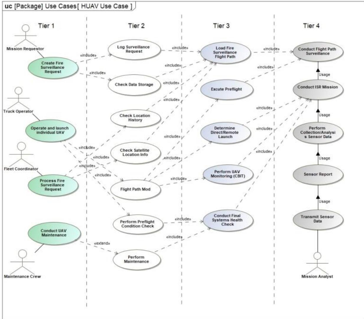
Figure 13: H-UAV Use Case Diagram
