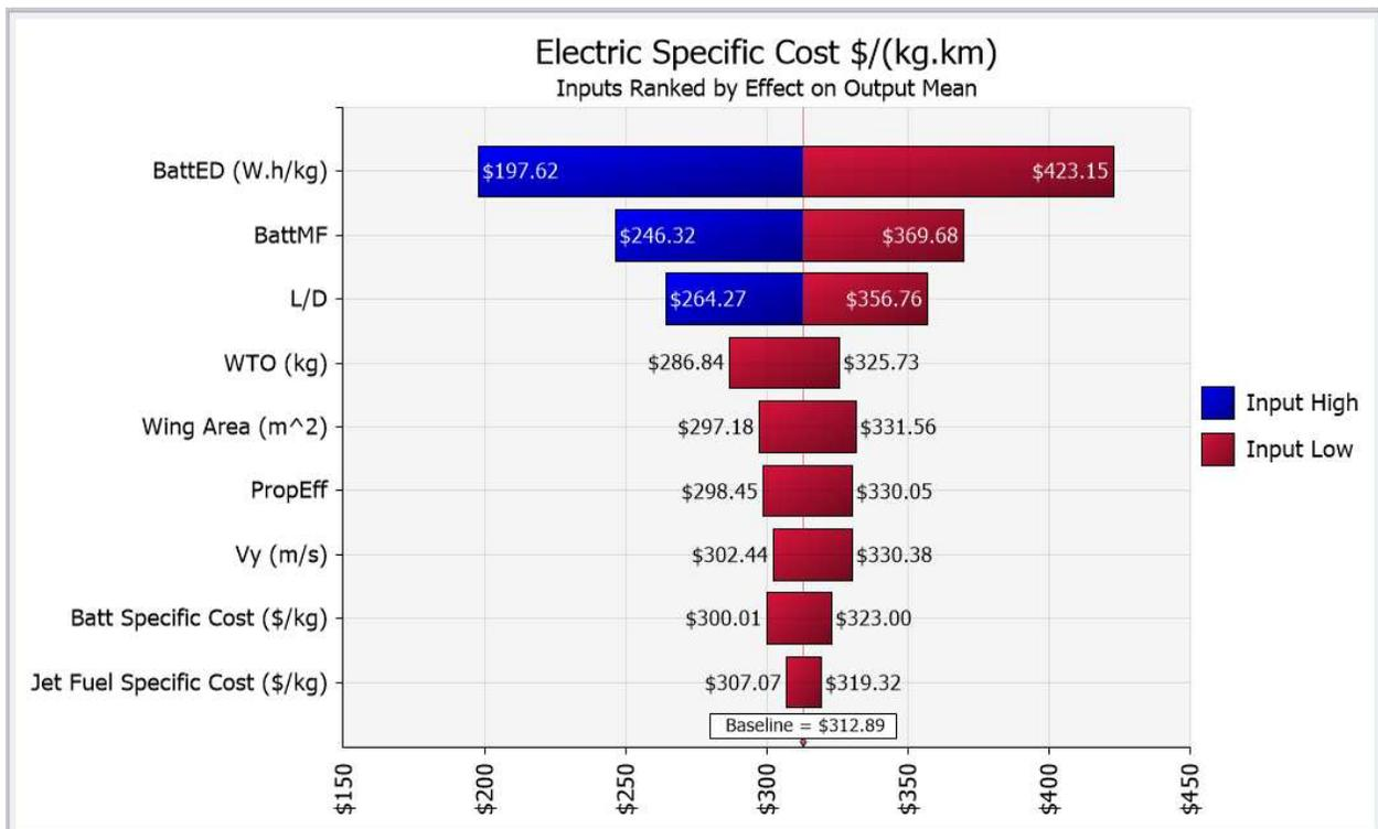
**Figure 43:** Tornado chart of specific cost drivers for the E-UAV (fully electric)
