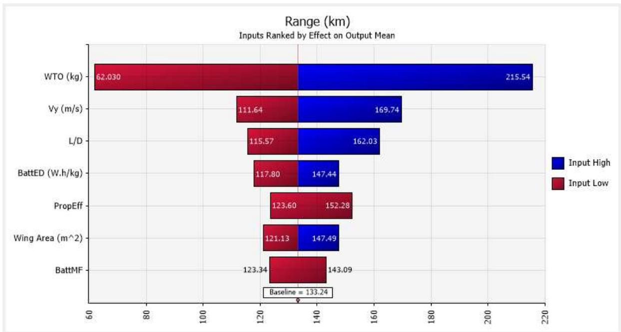
**Figure 37:** Tornado chart ranking the biggest design drivers for range of H-UAV
