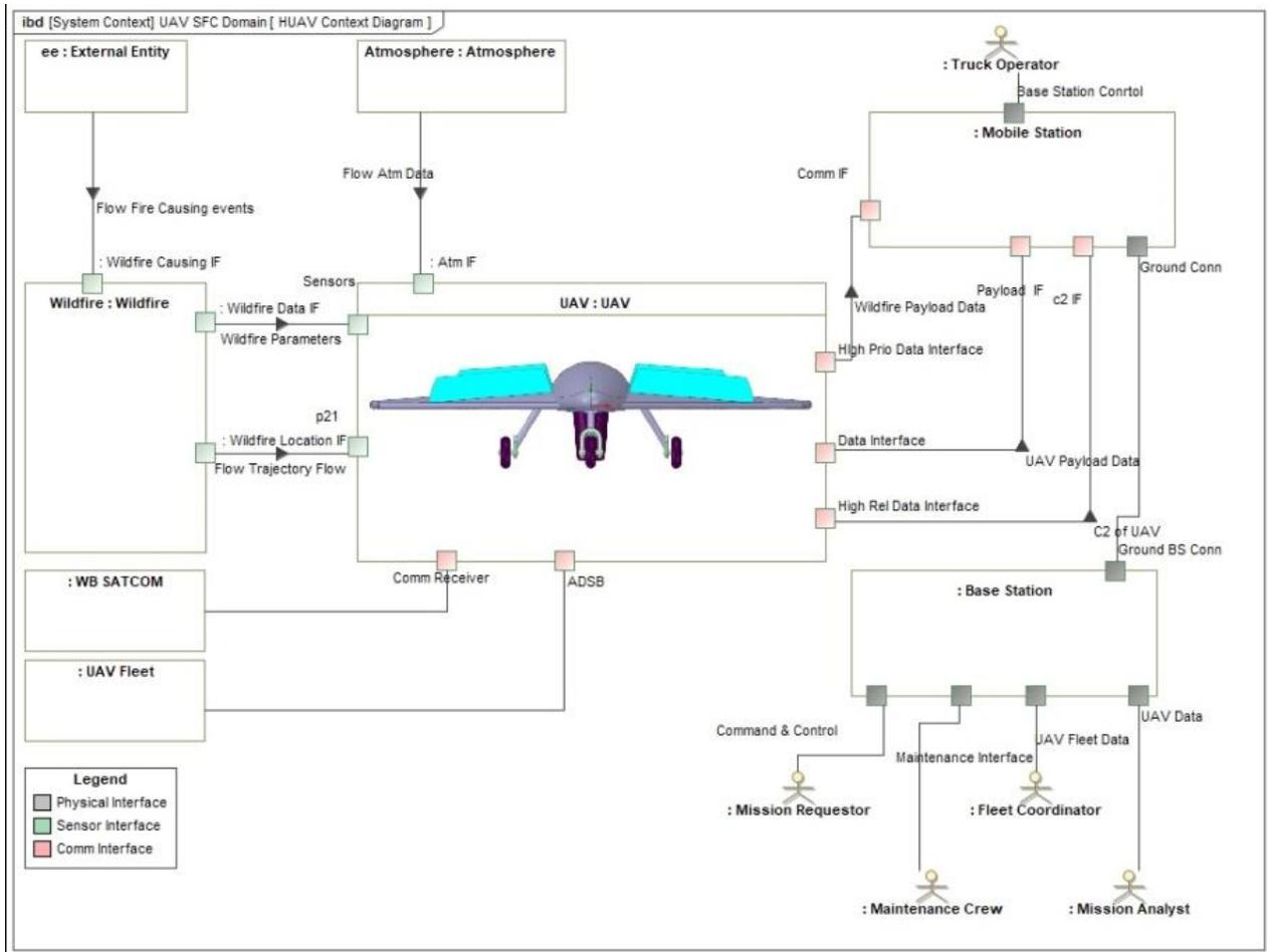
Figure 27: H-UAV Context Diagram
