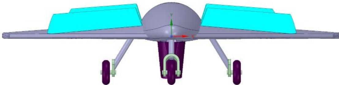
Figure 23: H-UAV Landing Configuration
