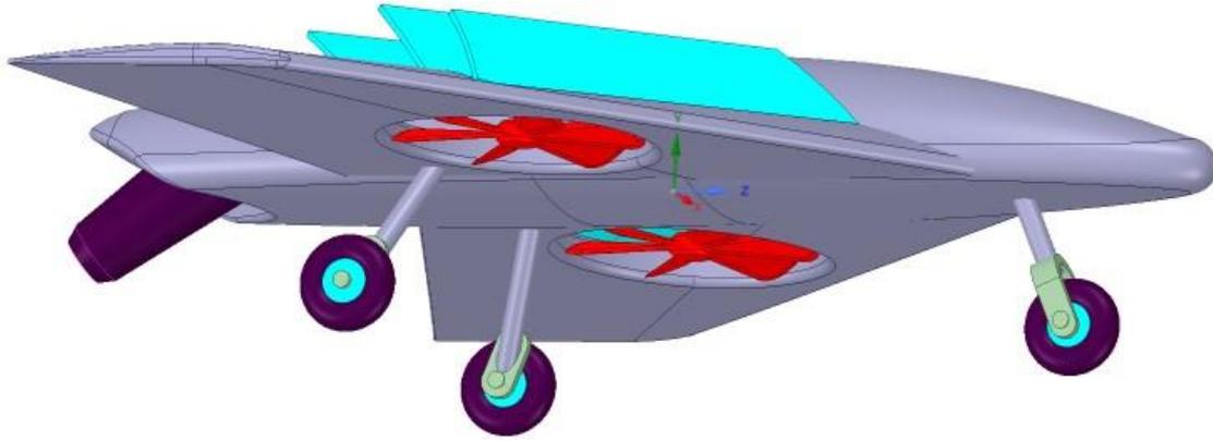
**Figure 32:** H-UAV Concept - Hybrid Propulsion
