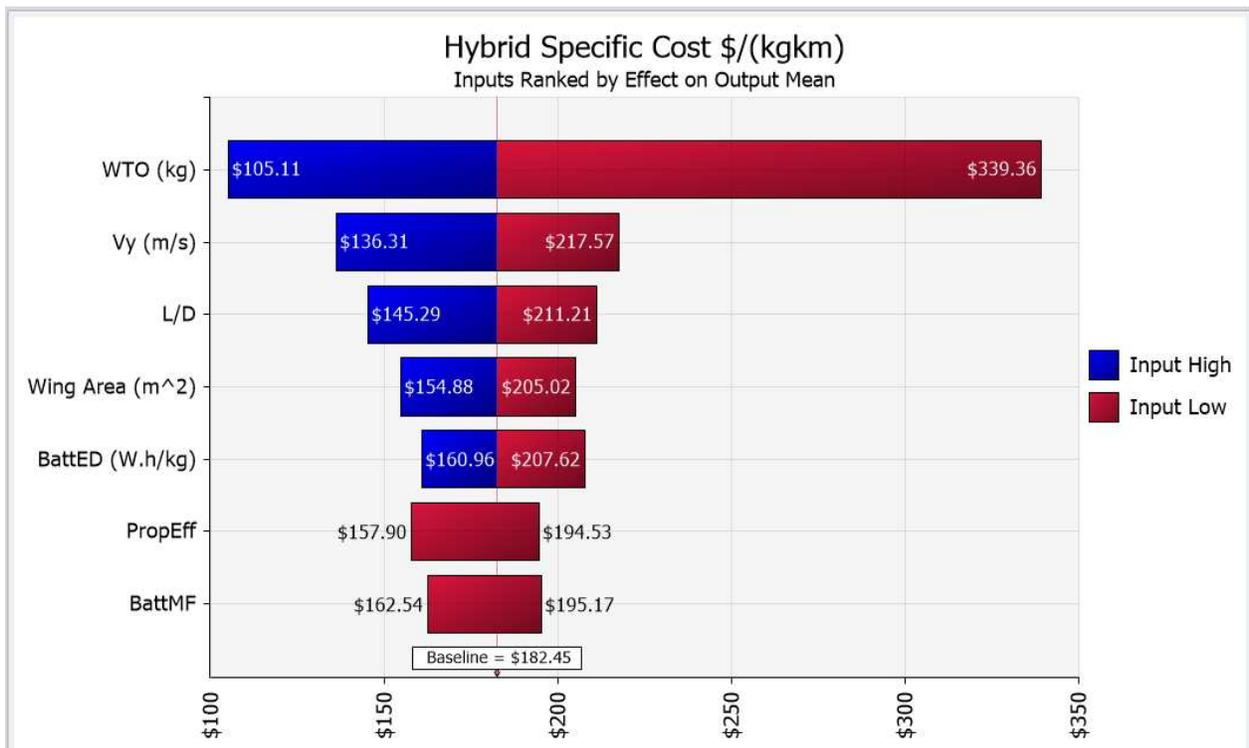
**Figure 44:** Tornado Chart of specific cost drivers for H-UAV (Hybrid Electric /Gas turbine)
