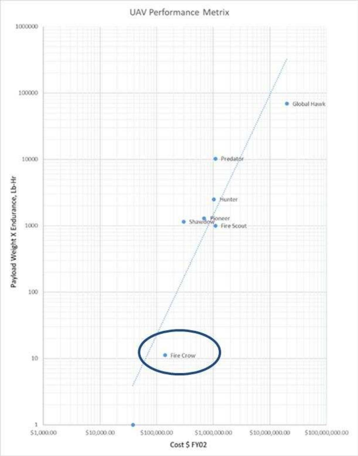
Figure 46: Comparison of H-UAV (Fire Crow) with other UAVs in literature
