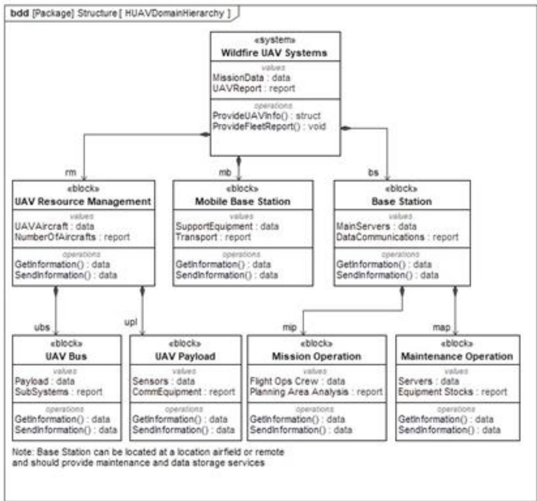
**Figure 9:** Fire Detection and Communication System Block Definition Diagram
