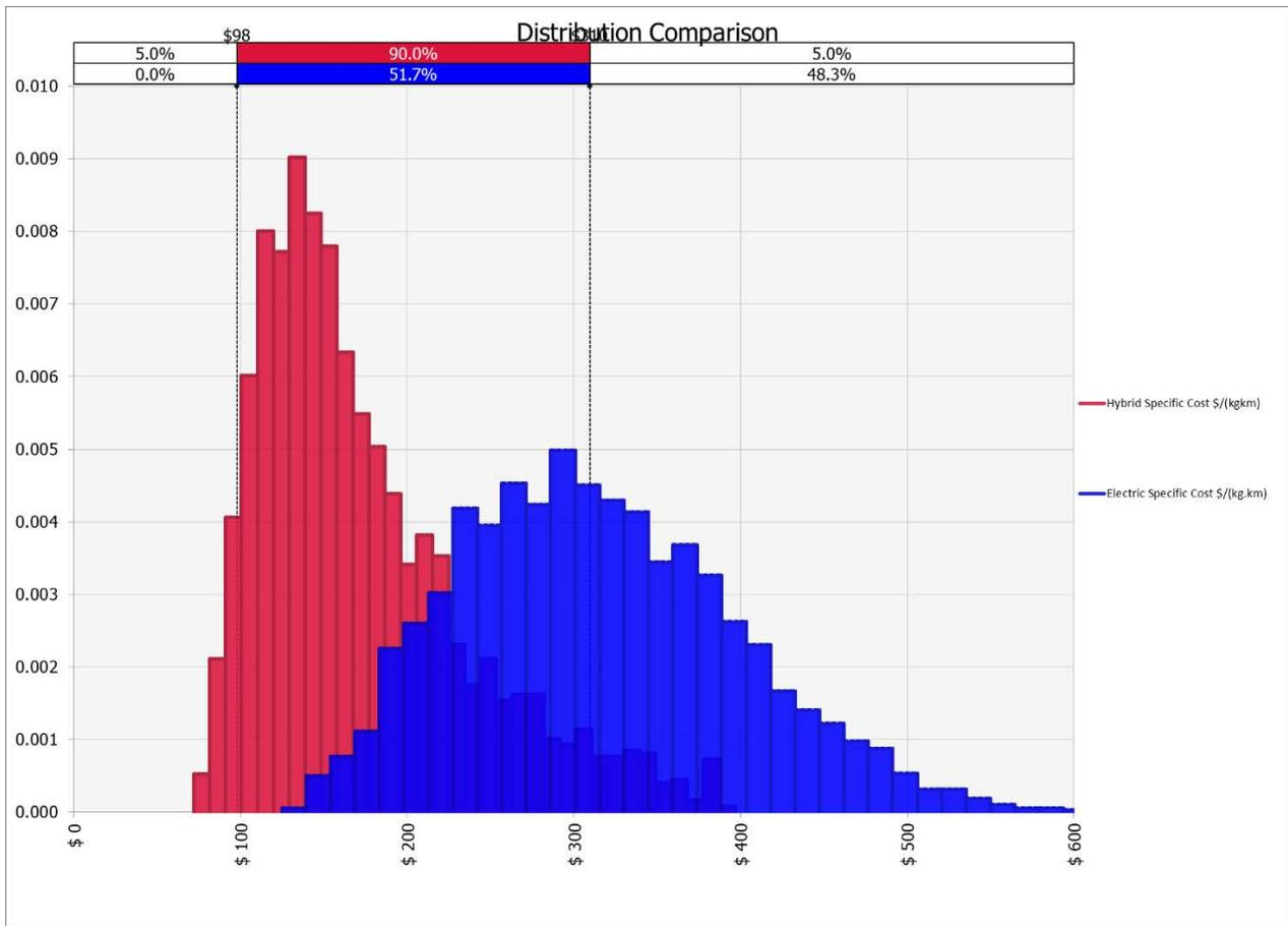
**Figure 25: H-UAV Specific Cost Comparison**
