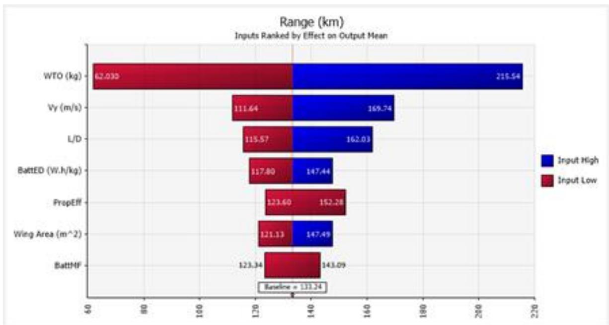
**Figure 20:** Tornado chart ranking the biggest design drivers for range of H-UAV
