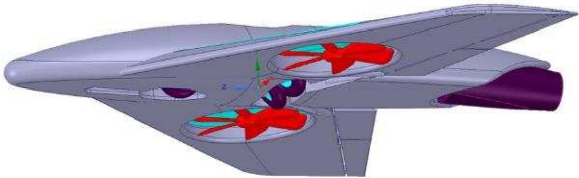
**Figure 41:** 1<sup>st</sup> Gen Optimal Design in Dash and Loiter Configuration
