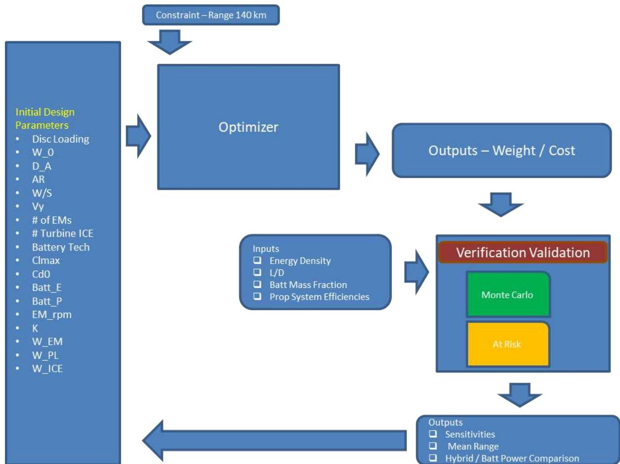
**Figure 34:** Optimizer wrapped inside a Monte Carlo Loop (Executable Model)
