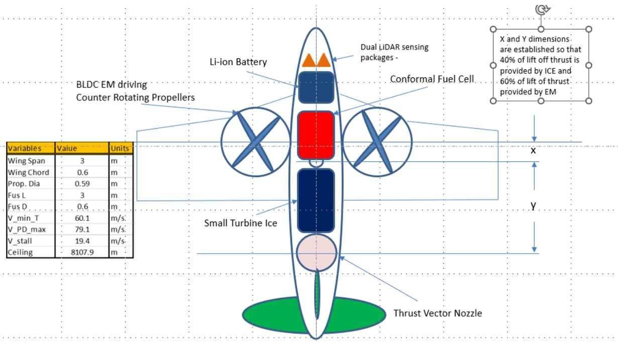
Figure 22: Initial H-UAV System Layout
