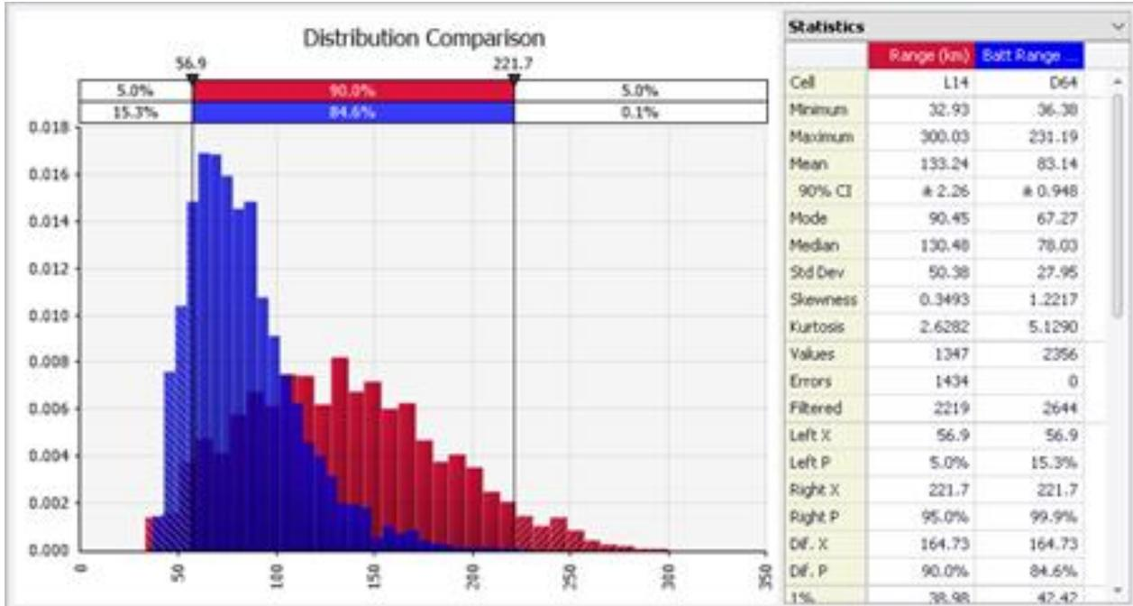
**Figure 36:** Range comparison between Fully Electric and Hybrid Electric/Gas turbine UAV
