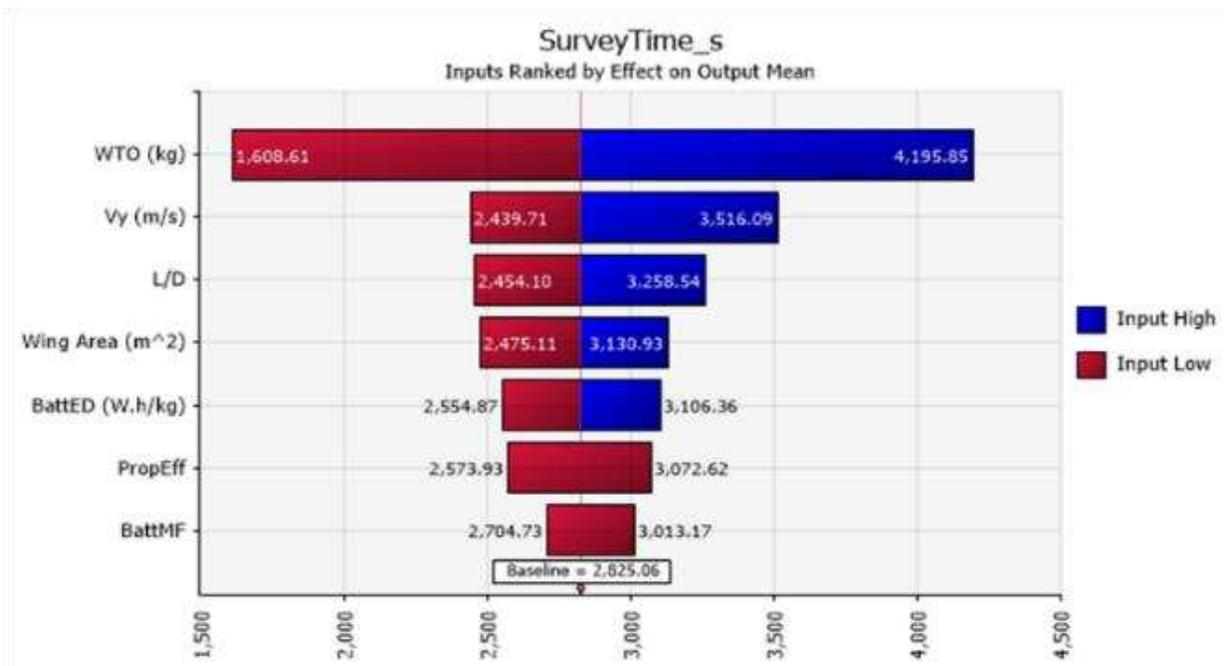
**Figure 47:** Tornado Chart of Survey Time for the H-UAV
