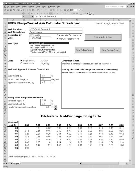
Figure 1. Example of Weir Calculator Spreadsheet.
