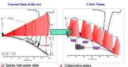
☐ Sensing gap: Earth curvature effects prevent 72% of the troposphere below 1 km from
