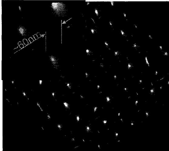
Figure 3.26. Fabricated array of holes patterned in PMMA by double exposure with a Lloyd's mirror configuration,  $\alpha = \pi/2$  and low ( $110\text{mJ}/\text{cm}^2$ , 40+40 laser shots) photon dose showing in details 60nm FWHM holes.
